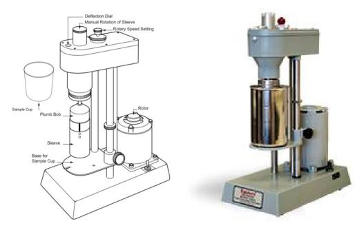
Figure 2. Fann rotary viscometer.
