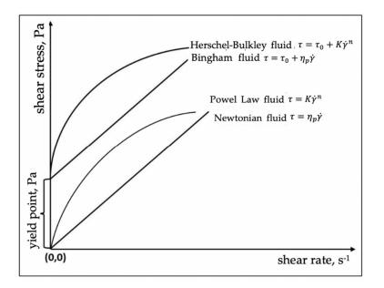
Figure 1. Flow curves of fluids obeying different flow models.
