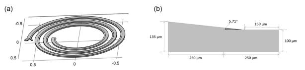
**Figure 1.** (a) Tilted top view of the spiral design with dimensions in cm. (b) Cross-sectional dimensions of the spiral geometry composed of a right-angled trapezoid and a rectangle.
