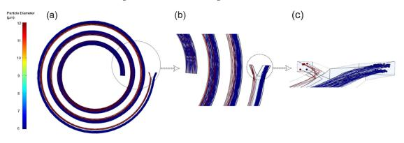
**Figure 4.** (a) Particle diameter differentiation inside the 135  $\mu$ m height spiral; (b) zoomed-in view on particle trajectory reaching the outlets; (c) zoomed-in view on the two outlets with clear particle separation.
