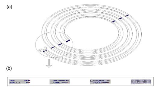
**Figure 6.** (**a**) Seven vertically-cut planes in the 150 μm height spiral. (**b**) Zoomed-in view on the left side of the microchannel showing scattered particles at each spiral turn.
