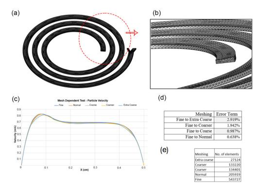
**Figure 2.** (a) Top view of the meshed spiral geometry. (b) Zoomed-in view of the tetrahedral elements. (c) Mesh-dependent test based on the velocity (m/s) at a line located just before the outlet. (d) Mesh errors in comparison to the fine mesh. (e) Number of tetrahedral elements in the mesh-dependent analysis against meshing type.
