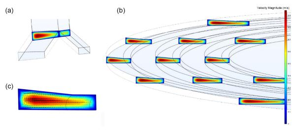
**Figure 3.** (a) Velocity contours normal to the fluid flow at the two outlets and (b) at different selected horizontal planes of the spiral geometry. (c) Normal velocity vectors at a random vertically cut slice.
