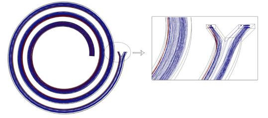
**Figure 5.** Particle separation inside the 120  $\mu$ m height spiral with a zoomed-in view on the two outlets showing mixed particle types.
