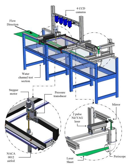
(SPHERICEL<sup>®</sup>, Potters Industries, Malvern, PA, USA). The laser beam was focused into a thin sheet and directed upstream by a mirror and a submerged periscope.
