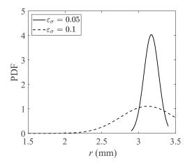
**Figure 11.** Probability density function of boundary radius for detected vortices based on 100 simulations at  $\varepsilon_{\sigma}$  values of 0.05 and 0.1, i.e., 5% and 10% noise, respectively.
