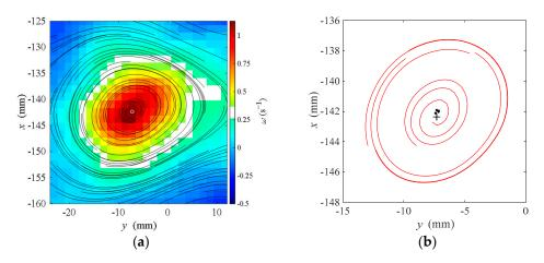
**Figure 16.** Illustration of a sample vortex along with a locally computed velocity field centered on the vortex core. The velocity field is calculated in a moving reference frame matching the drift velocity of the sample vortex. In (**a**), streamlines generated from the velocity field overlay the local vorticity field, and (**b**) highlights five streamlines meeting WA criteria, along with cluster points (black), determined via the CSL method, denoted by a black '+' symbol.
