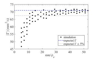
**Figure 8.** Circulation data are excluded for cases with  $nm/\emptyset_v < 5$ , as rejected by the WA method. The computed circulation pertains to the core region circulation, representing circulation induced within the vortex boundaries ( $-r_v \le r \le r_v$ ).
