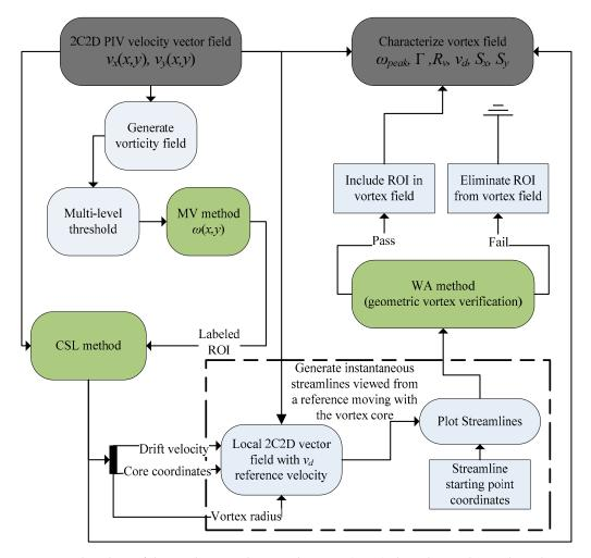
**Figure 4.** Flowchart of the combinatorial vortex detection (CVD) algorithm, utilizing three detection methods, MV, CSL and WA (green boxes), to process a 2C2D velocity vector field and generate characterized vortex data.
