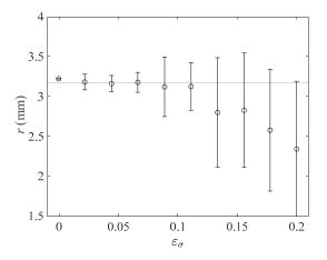
**Figure 10.** Mean radius computed by the CVD for 100 simulations at various noise levels, along with standard deviation error bars.
