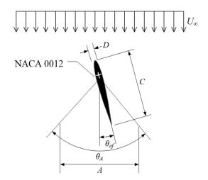
**Figure 13.** Representation of the aluminum airfoil, a continuous extrusion with an NACA 0012 crosssectional shape and a chord length (*C*) of 75 mm. The figure also illustrates the motion parameters, including pitch oscillations, enabled by a sturdy shaft driven by a stepper motor passing through the airfoil's aerodynamic center.
