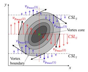
**Figure 2.** Schematic representation of the cross-sectional lines (CSL) procedure with four concentric ellipses illustrating vorticity contours and the vortex core indicated by an ' $\times$ '.
