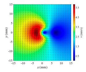
**Figure 5.** Simulated velocity vector field ( $200 \times 200$  resolution) with velocity magnitude represented by a color map, showing every 6th vector.
