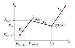
**Figure 3.** Computation of angle  $\alpha_{w,i}$  on streamline  $S_k$  for the winding angle algorithm.
