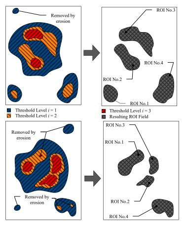
**Figure 1.** Schematic illustrating the application of a multilevel threshold technique for identifying vortices in two vorticity fields. (**left**): indexed images with levels *i* = 1, 2, and 3. (**right**): corresponding desired ROI maps for vortex extraction.
