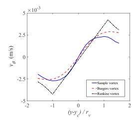
**Figure 18.** Comparison of circumferential velocity profiles for the sample vortex, a Rankine vortex, and a Burgers vortex.
