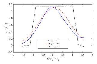
**Figure 17.** Vorticity distribution profiles of an identified vortex, showing the vorticity plotted against the dimensionless radius along a constant *y* line traversing the vortex core. Additionally, vorticity profiles for ideal Burgers and Rankine vortices are included, sharing the same peak vorticity and radii as computed by the CSL algorithm.
