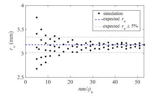
**Figure 7.** Vortex radius variations calculated by the CVD algorithm for different  $nm/\emptyset_v$  values, compared with the expected radius ( $r_v = 3.18 \text{ mm} \pm 5\%$ ) in the Burgers model. Vortices with  $nm/\emptyset_v < 5$  are disregarded. Discretization artifacts from the simulation are also evident.
