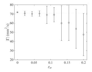
**Figure 9.** Mean circulation computed by the CVD for 100 simulations at various noise levels, along with standard deviation error bars.
