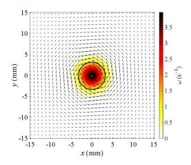
**Figure 6.** Simulated velocity vector field ( $200 \times 200$  resolution) with the freestream velocity ( $U_{\infty}$ ) subtracted, displaying every 6th vector, and featuring vorticity as a color map in the background.
