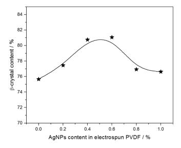
**Figure 4.** β-phase content of PVDF in the PVDF/AgNPs composites (line added to guide the eye).
