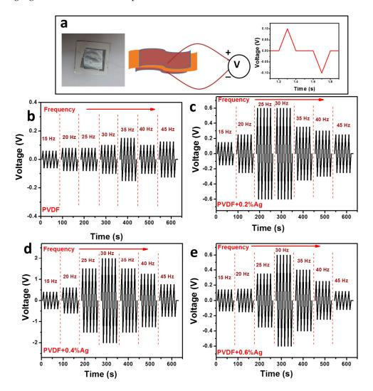
**Figure 11.** (a) Sample used for the piezoelectric experiment and its schematic representation. Voltage versus time graphs at different vibrating frequencies (b) Pure PVDF; (c) PVDF + 0.2% Ag; (d) PVDF + 0.4% Ag; and (e) PVDF + 0.6% Ag nanocomposites.
