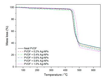
Figure 6. TGA curves of PVDF and the PVDF/AgNPs composites.
