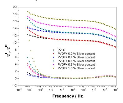
**Figure 8.** Dielectric permittivity storage ( $\varepsilon'$ ) (closed symbols) and loss ( $\varepsilon''$ ) (open symbols) of the electrospun PVDF/AgNPs composite fiber mats having different compositions at 20 °C.
