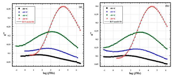
**Figure 9.**  $\varepsilon''$  vs. logf spectra for the electrospun (a) PVDF and (b) PVDF/0.4% AgNPs samples within the  $\beta$ -relaxation temperature range. Lines represent the HN equation fits to the spectra.
