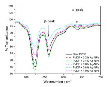
$\textbf{Figure 3.} \ \ \textbf{FTIR} \ \ \textbf{spectra of the PVDF/AgNPs} \ \ \textbf{electrospun nanocomposite fibers prepared in this investigation}.$
