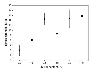
**Figure 7.** Tensile strengths of PVDF/AgNPs composites as function of AgNPs content. Black squares represent the mean values of the tensile strength while lines represent the standard error of these values.
