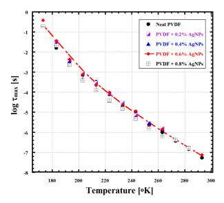
**Figure 10.** VFTH plots for the *β*-relaxation of the electrospun PVDF/AgNPs composite fiber mats having different compositions. The dashed line represents the VFTH equation fit to the data for the PVDF + 0.6% AgNPs sample.
