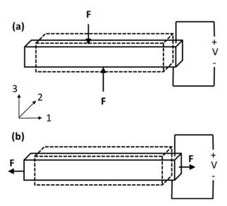
**Figure 5.** Schematic view of piezoelectric beams generating voltage in (**a**) 33 mode, and (**b**) 31 mode. The dashed outline represents the original shape; the solid outline represents the deformed shape.
