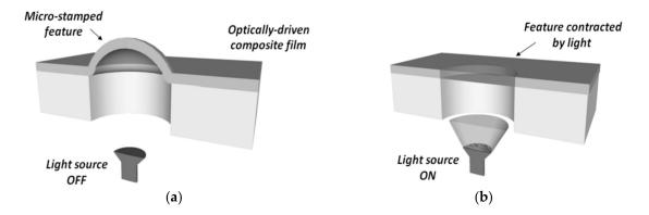
**Figure 3.** Schematic concept of carbon nanotube (CNT) composite film driven by the light source to form "blister" shape and flat shape for actuation. (a) Default state: the light source is OFF. The feature is a high-relief dot; (b) the feature flattens when it is light-actuated. This actuation is reversible when the light is turned off. Adapted from [52].
