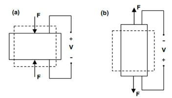
**Figure 4.** Schematic diagrams showing the piezoelectric effect. The dashed outline represents the object's original shape; the solid outline represents the object's deformed shape-contracting (a) and expanding (b).
