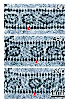
**Figure 10.** Aberration-corrected TEM images of  $D_{5d}$ -C<sub>80</sub> fullerene molecules inside (18,1) SWNT, from work by Suenaga et al. Reproduced with permission from [78]. American Chemical Society, 2007. Triangles indicate encapsulated molecule undergoing orientational changes.
