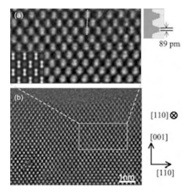
**Figure 13.** Aberration corrected TEM image of diamond projected along <110>. (**a**) Magnified image. (**b**) Full image. An intensity profile is shown at upper right and a simulated image is shown as an insert in (**a**). From work by Hosokawa et al. Reproduced with permission from [98]. Oxford University Press, 2013.
