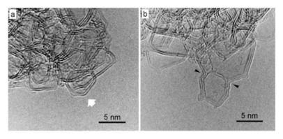
**Figure 7.** (a) Micrograph showing closed structure in polyvinylidene chloride (PVDC)-derived carbon heated at 2600 °C; (b) another micrograph of same sample, with arrows showing regions of negative curvature. From work by Harris and Tsang. Reproduced with permission from [61]. Taylor & Francis, 1997.
