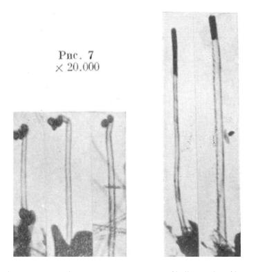
**Figure 1.** Very early transmission electron microscopy images of hollow carbon filaments. Reproduced with permission from [22]. Nauka Publishers, 1952.
