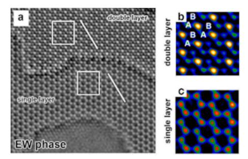
**Figure 12.** (a) Exit wave function (EW) reconstruction TEM image of single and bilayer graphene sheets; (b,c) Higher magnification colourised images from parts of single and bilayer regions. Reproduced with permission from [94]. Elsevier, 2011.
