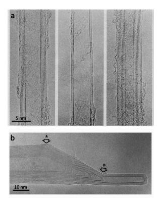
**Figure 4.** (a) Some of Iijima's first images of multiwalled nanotubes. Reproduced with permission from [49]. Springer Nature, 1991; (b) Multiwalled nanotube cap. "A" indicates position of single pentagon; "B" indicates probable position of single heptagon. Reproduced with permission from [51]. Springer Nature, 1992.
