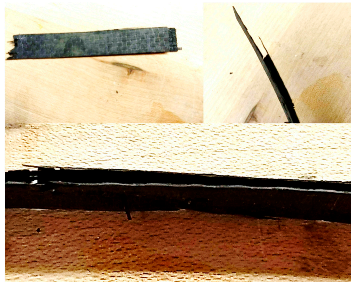
Figure 7. Delamination in composites based on carbon fibers and Bucky paper without ZnO nanorods.
