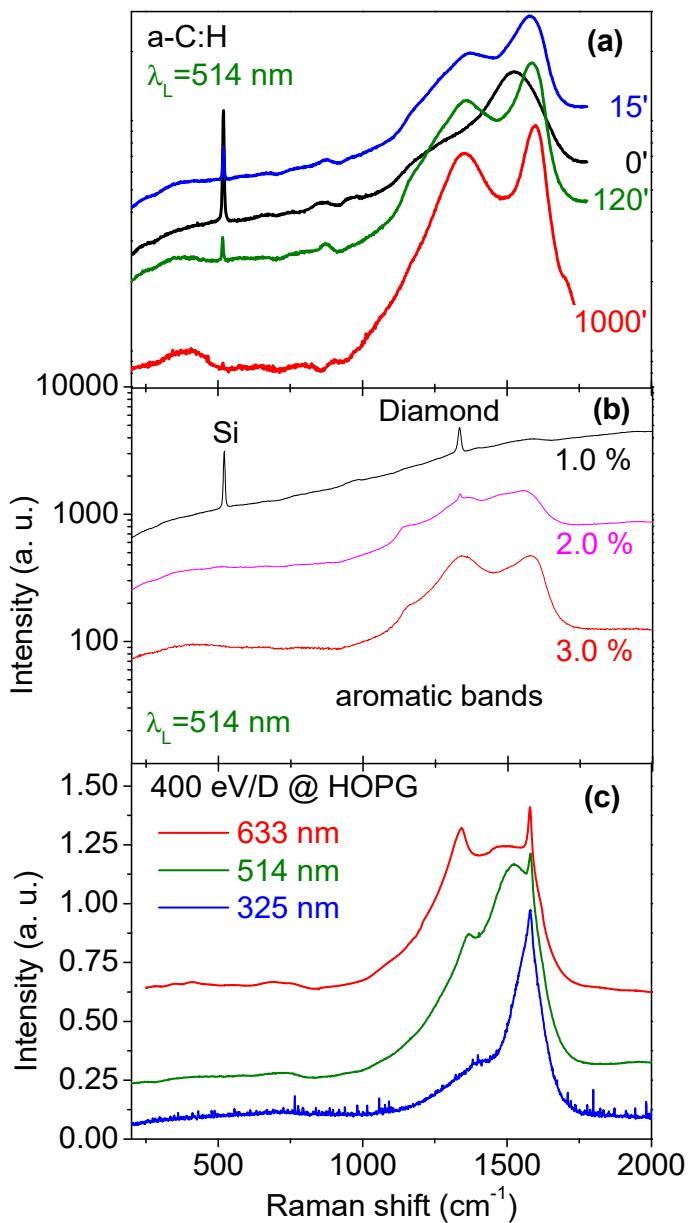
**Figure S2.** Multi-wavelength Raman spectra without base line subtraction. (a) heated a-C:H samples, (b) as-grown diamond films, (c) bombarded graphite (400 eV/D).
