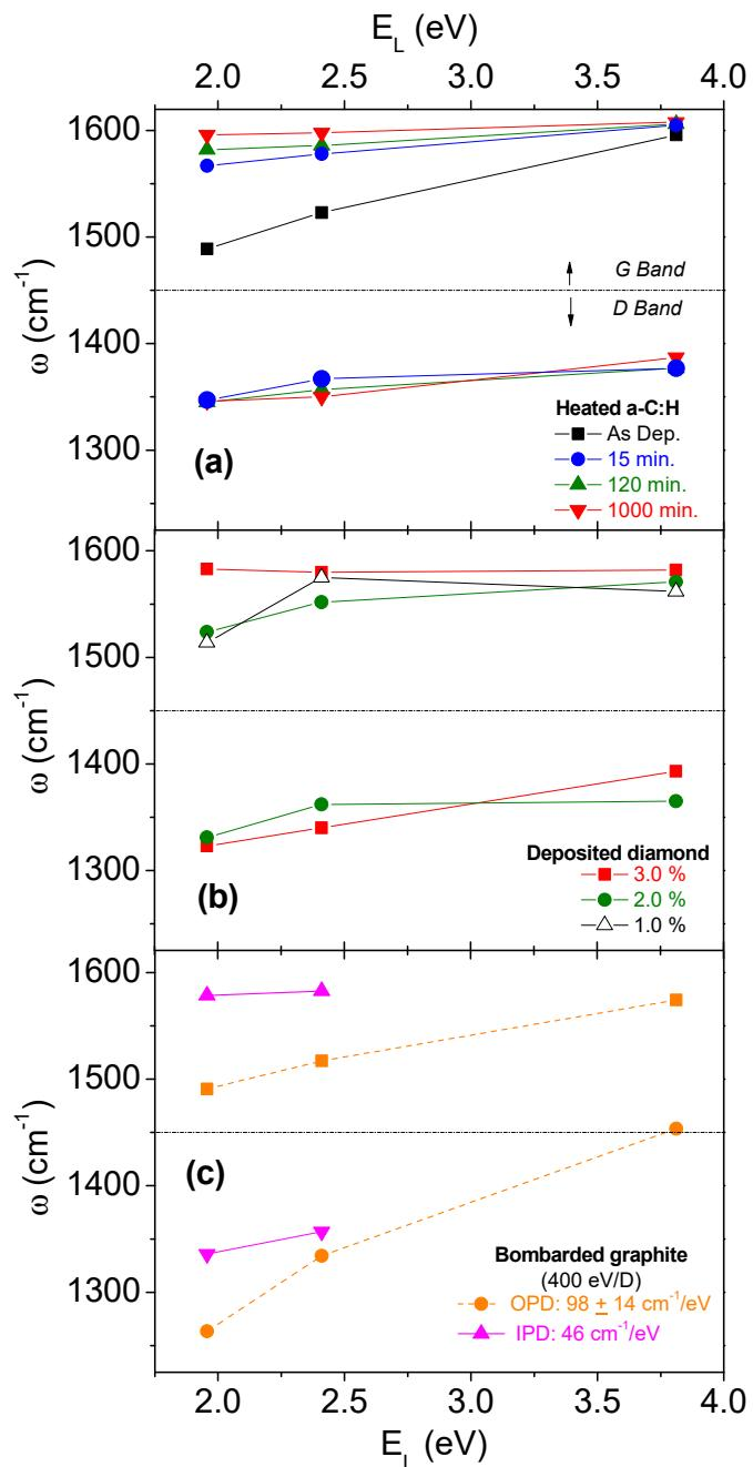
**Figure S1.** D and G band dispersion. (a) heated a-C:H samples, (b) as-grown diamond films, (c) bombarded graphite (400 eV/D).
