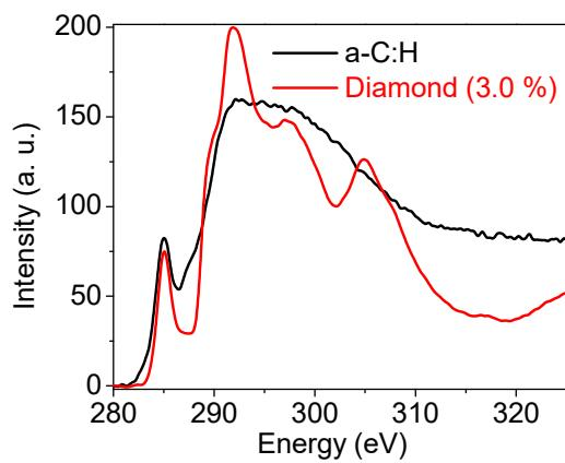
**Figure S3.** EELS spectra of as deposited a-C:H sample, and as-grown diamond film. Methodology to obtain  $\text{sp}^2/\text{sp}^3$  ratio is explained in Lajaunie et al (2017).
