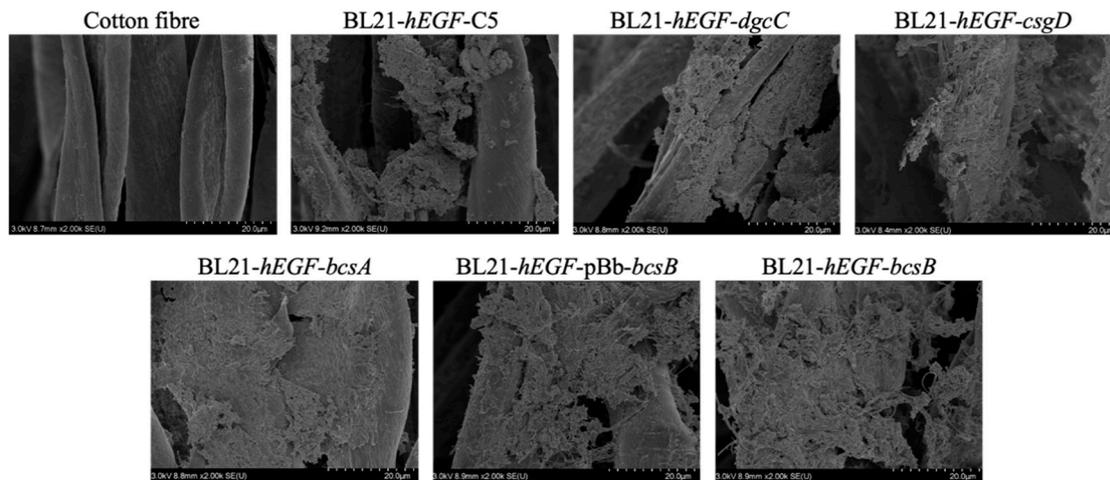
**Figure 9.** SEM image of the carrier in immobilized continuous fermentation. Biofilm on the carrier after immobilized continuous fermentation; image taken by SEM. Scale bar, 20 µm.
