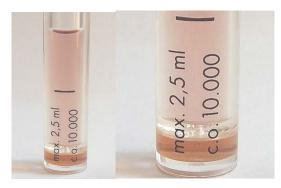
**Figure 4.** Centrisart filter system with a 10 kDa cutoff in two magnifications separating filtrate (top); and concentrate (bottom) of an ABTS derivative catalyzed by European beech sapwood.
