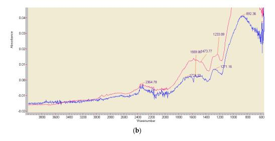
**Figure 8.** FT-IR analyses of the red ABTS derivatives obtained by  $K_2O_8S_2$  oxidation (**a**), and of the product generated by enzymatically active beech wood chips (**b**) (red curve), paired with an ABTS-free reference sample (blue curve). The major peak at 858.86 cm<sup>-1</sup> is not shown.
