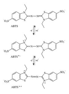
**Figure 1.** Oxidation of the heterocyclic ABTS molecule (shown as a dianion) to ABTS<sup>2+</sup> by two consecutive electron abstractions.
