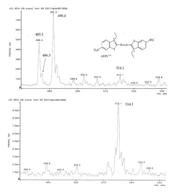
**Figure 6.** LC-MS chromatograms in the positive mode of a non-purified ABTS derivative with the protonated dianion of  $ABTS^{(2+)}$  (m/z 514.1), its deethylated ( $C_2H_5$ ) form recompleted by methyl groups ( $CH_3$ , m/z 486.3), and major ABTS moieties.
