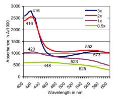
**Figure 3.** Doses of  $H_2O_2$  rising in the range of  $0.5-3\times$  alter the positions of absorbance peaks of the ABTS derivative catalyzed by beech sapwood. In comparable tests with birch sapwood, the final peak moved with the rising  $H_2O_2$  doses from  $A_{537}$  to  $A_{548}$ . Dose " $1\times$ " refers to the  $H_2O_2$  concentration given in Section 2.2.
