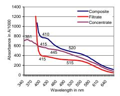
**Figure 5.** Filtration against a 10-kDa cutoff: Positions of absorbance peaks of the composite ABTS derivative as catalyzed by beech sapwood, of the filtrate  $\leq$  10 kDa, and the concentrate  $\geq$  10 kDa.
