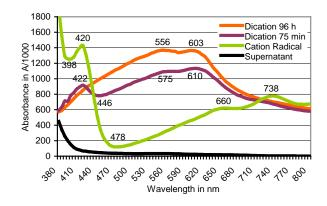
**Figure 7.** Oxidation of ABTS with potassium peroxodisulfate as followed by scanning spectrophotometry. The peaks at  $\lambda = 420/660/738$  nm shown by the green ABTS<sup>•+</sup> oxidation state (reaction time, 10 min) are replaced by peaks around 556/603 nm of the deep lilac and flocculent (insoluble) reaction product (reaction time, 75 min to 96 h) which precipitates in the colorless supernatant of non-depleted K<sub>2</sub>O<sub>8</sub>S<sub>2</sub> solution of pH 2.15.
