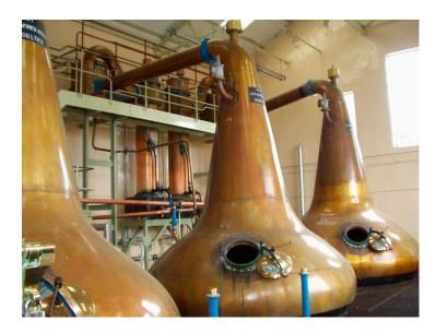
Figure 22. A typical pot still employed for the batch distillation of malt whisky.
