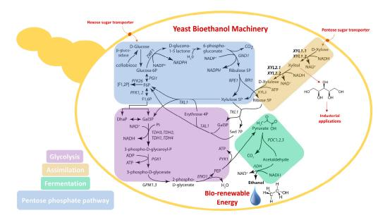
Figure 4. Model for bioethanol production using yeast fermentation machinery.
