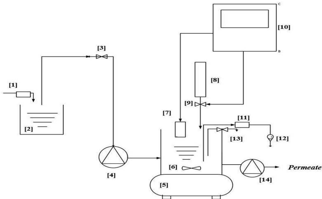
**Figure 1.** Schematic diagram of the continuous culture reactor (CSTR) (1) Air Filter (2) Feed vessel (3) valve (4) Feed pump (5) Magnetic stirrer plate (6) Stirring bar (7) pH probe (8) Alkali reservoir (9) valve (10) pH controller (11) Air filter (12) Rotameter (13) Sampling port (14) Effluent pump.
