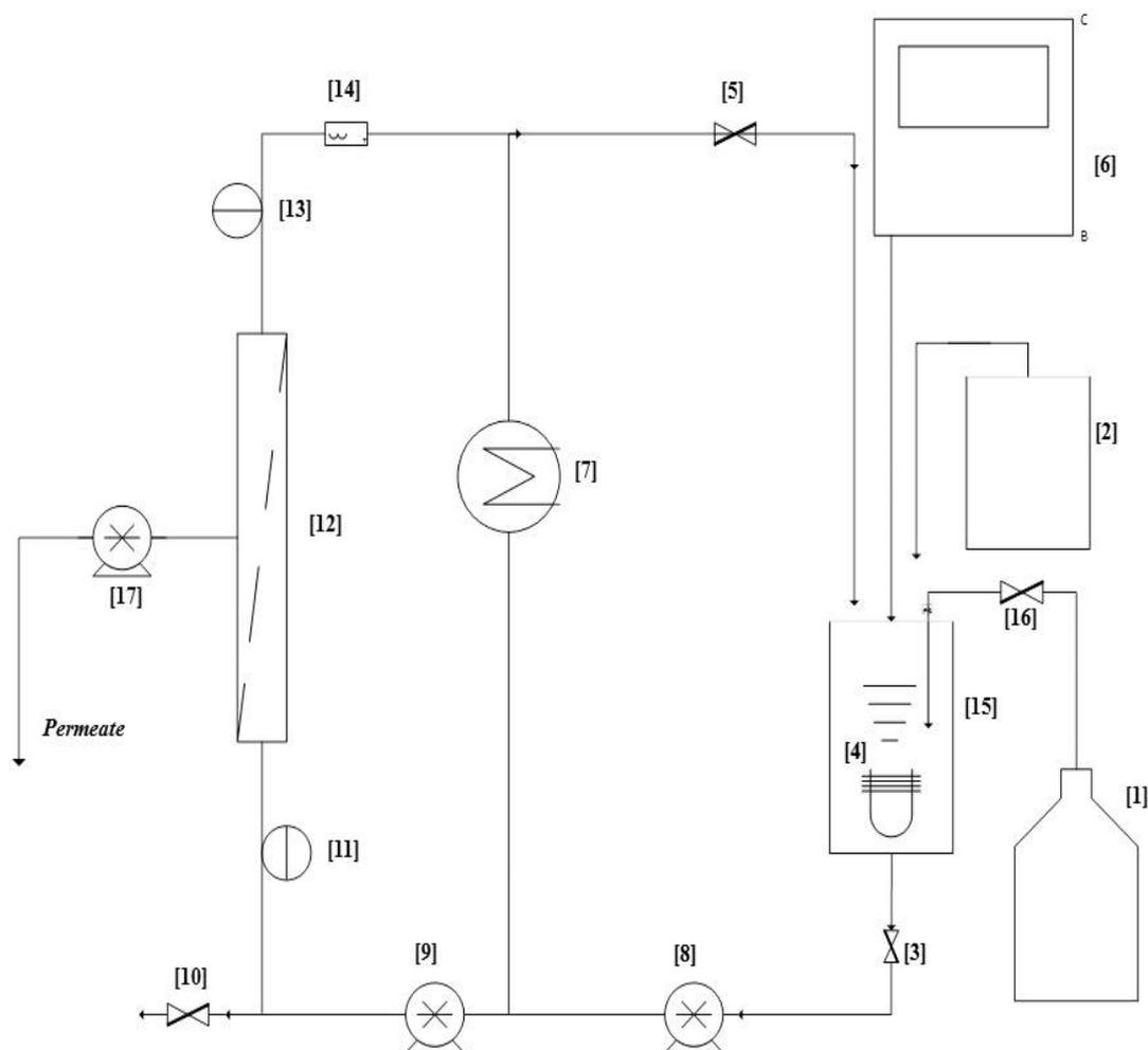
**Figure 2.** Schematic diagram of the membrane bioreactor (MBR) (1) Nitrogen gas supply (2) Feed vessel (3) diaphragm valve (4) Coils (5) Diaphragm valve (6) control panel(including level and temperature controller) (7) Heat exchanger (8) Feed pump (9) recirculation pump (10) drain valve (11) Pressure gauge (12) Hollow fiber module (13) Pressure gauge (14)Thermocouple (15) reaction vessel (16) feed valve (17) peristaltic pump.
