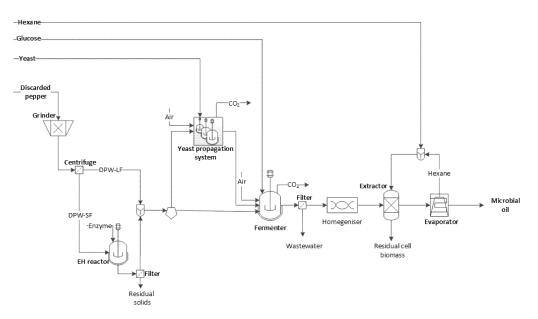
Figure 1. Simplified diagram of the microbial oil production plant based on discarded peppers.
