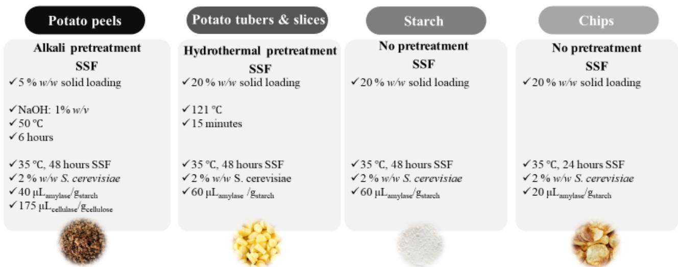
Figure 9. Optimum conditions for bioethanol production from potato chips industry waste.
