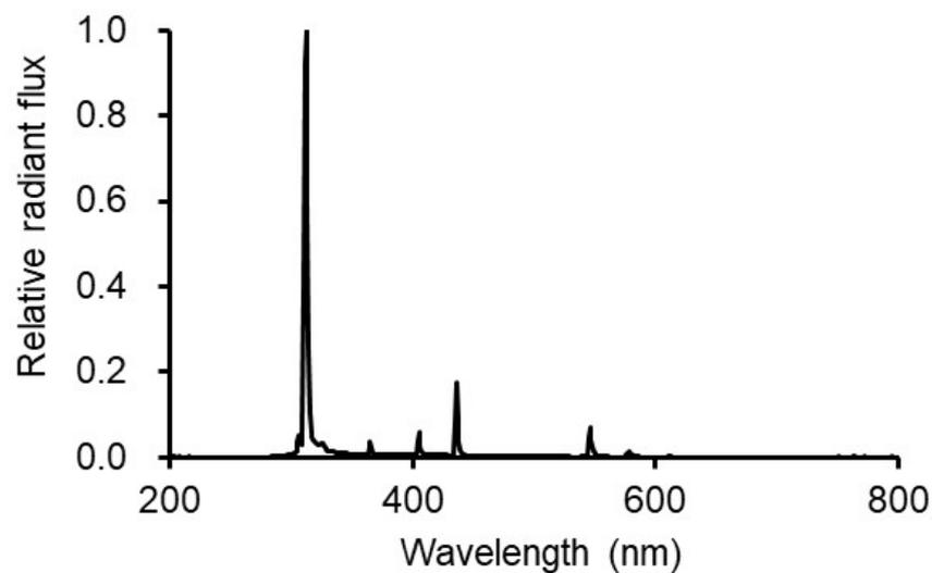
**Figure 1.** Spectral radiant flux of the UV-B lamps used in this study (TL20W/01 RS; Philips, Hamburg, Germany).
