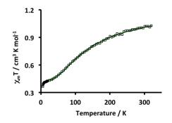
**Figure 4.** Plot of  $\chi_m T$  vs. *T* for **5**. Squares represent the experimental data points and the green curve represents the best fit to the experimental data (best fit parameters are provided in the text). External field 5000 Oe.
