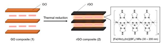
**Figure 1.** Schematic illustration of pressure effects in graphene oxide (GO)/ reduced graphene oxide (rGO) layers incorporating [Fe(Htrz)<sub>2</sub>(trz)](BF<sub>4</sub>) nanorods (NRs).
