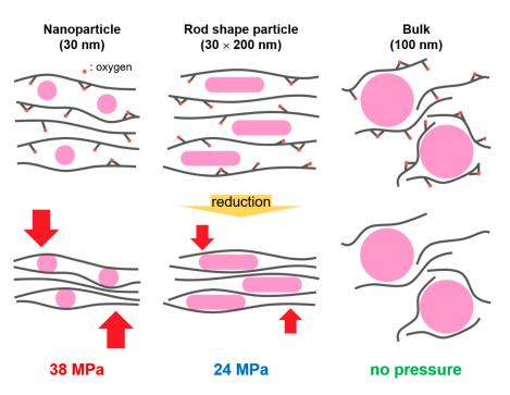
**Figure 5.** Schematic illustration of the pressure effects with incorporated particle size and shape dependency in the GO/rGO layers.
