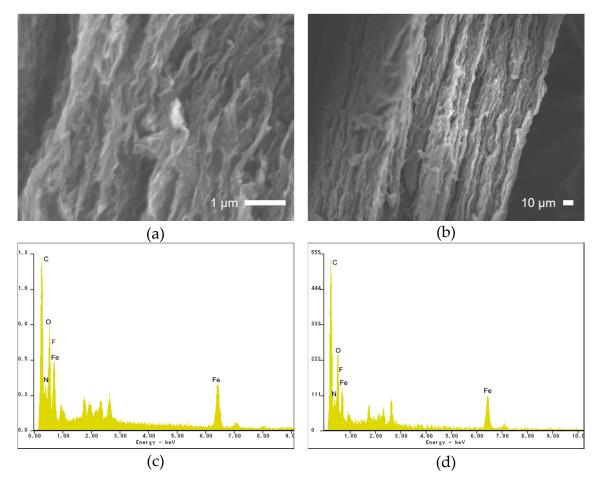
**Figure 2.** Scanning electron microscopy (SEM) images of (**a**) composite **1** and (**b**) composite **2**. SEM-energy dispersive X-ray spectroscopy (SEM-EDX) results for (**c**) composite **1** and (**d**) composite **2**.
