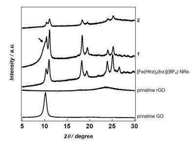
**Figure 3.** Powder X-ray diffraction (PXRD) patterns for pristine GO, pristine rGO, [Fe(Htrz)<sub>2</sub>(trz)](BF<sub>4</sub>) NRs, composite **1**, and composite **2**.
