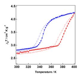
**Figure 4.**  $\chi_g T$  vs. *T* plots for composite **1** (heating: ( $\blacktriangle$ ); cooling: ( $\triangledown$ )) and composite **2** (heating: ( $\blacktriangle$ ); cooling: ( $\triangledown$ )).
