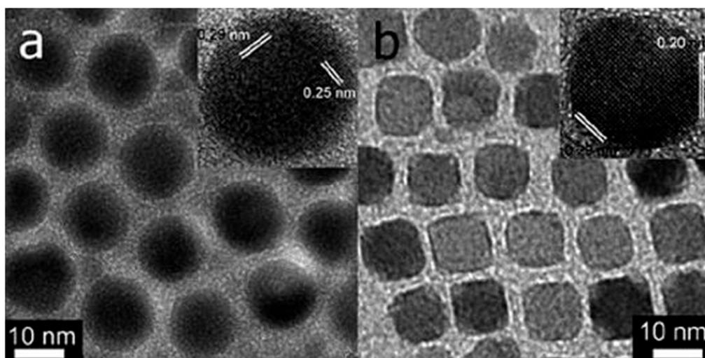
**Figure 2.** Transmission electron microscopy (HR TEM) images of monodisperse (a) nanosphere, (b) nanocubes by thermal decomposition method. Reprinted with permission from reference [21] Copyrights 2008, American Chemical Society.
