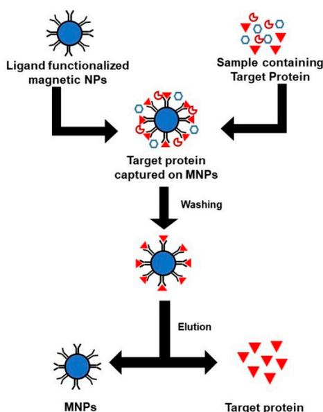
**Figure 5.** Schematic illustration of magnetic affinity separation of proteins.
