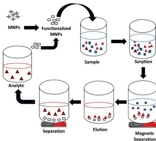
**Figure 4.** Schematic illustration of magnetic solid phase extraction.
