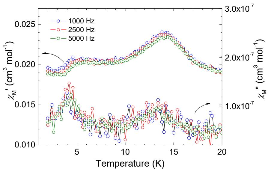
**Figure S13.**  $\chi'$  and  $\chi''$  plots of ac magnetic susceptibilities in a zero applied dc field and in an ac field of 3.5 Oe at the indicated frequencies for a powdered sample of compound **2**.
