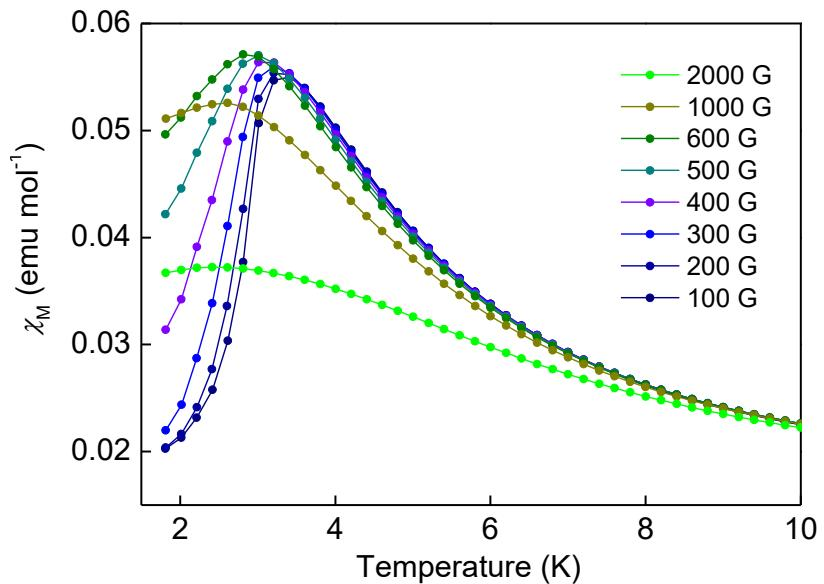
**Figure S8.** FC magnetization curves measured under different external fields for compound **1**.
