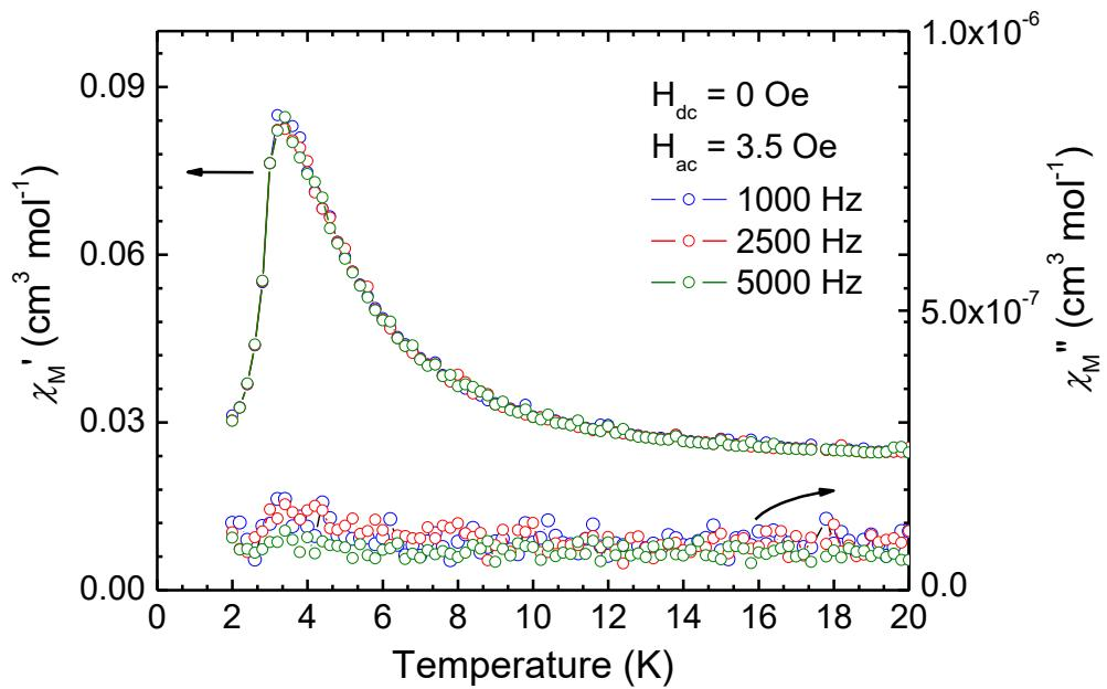
**Figure S6.**  $\chi'$  and  $\chi''$  plots of ac magnetic susceptibilities in a zero applied dc field and in an ac field of 3.5 G at the indicated frequencies for a powdered sample of compound **1**.
