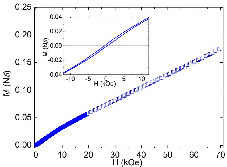
**Figure S14.** Field dependence of the magnetization of compound **2** (Co) at 2.0 K. The inset gives a blow-up of the hysteresis loop.
