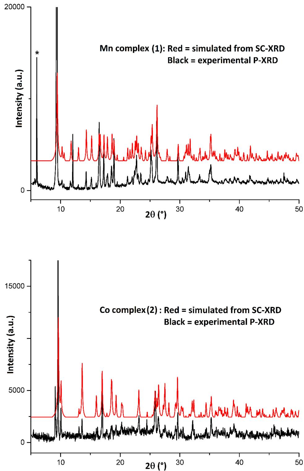
**Figure S1.** Experimental (black) and simulated (red) XRD powder patterns for complexes **1** (top) and **2** (bottom). Simulated patterns were generated using Mercury software (CCDC, see ref. 9 in main manuscript) with  $\lambda = 1.54 \text{ \AA}$  and the single-crystal structure refinements. In the pattern of **1**, the low-angle peak marked with an asterisk is probably due to the sample holder. A calculated baseline was subtracted in both experimental patterns.
