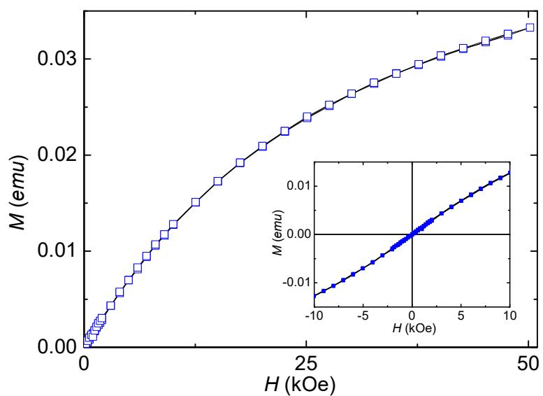
**Figure S17.** Field-dependent magnetization of the thermally decomposed compound **2** at 2.0 K. The inset gives a low field range of  $M$  vs  $H$ .
