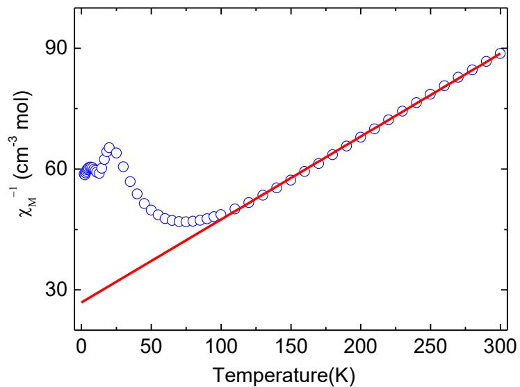
**Figure S12.** Plot of  $\chi_M^{-1}$  (circles) vs. temperature for a powdered sample of compound **2**. The solid line represents the best fit  $\chi_M^{-1}$  above 100 K with a Curie-Weiss law.
