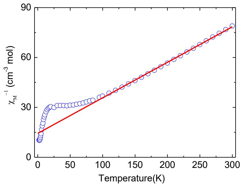
**Figure S3.** Plot of  $\chi_M^{-1}$ (circles) vs. temperature for a powdered sample of compound **1**. The solid line represents the best fit  $\chi_M^{-1}$  above 110 K with a Curie-Weiss law.
