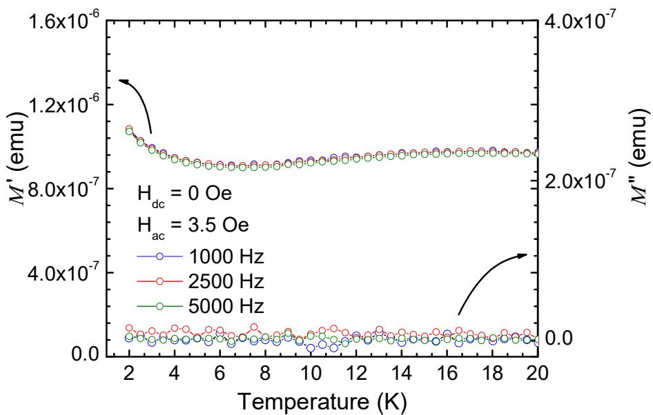
**Figure S18.** Plots of the temperature dependence of  $M'$  and  $M''$  of ac magnetic susceptibilities of thermal decomposed compound **2** in a zero applied dc field and in an ac field of 3.5 G at the indicated frequencies.
