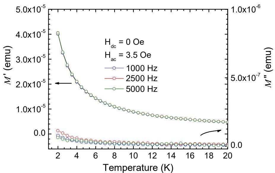
**Figure S15.** Plots of the temperature dependence of  $M'$  and  $M''$  of the ac magnetic susceptibilities of thermally decomposed compound **1** in a zero applied dc field and in an ac field of 3.5 Oe at the indicated frequencies.
