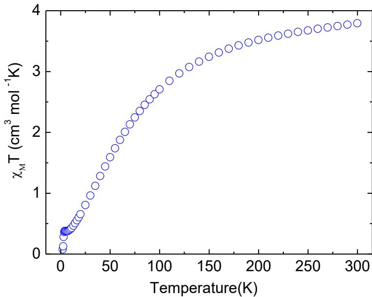
**Figure S4.** Plot of  $\chi_M T$  vs.  $T$  of powdered samples of compound **1** in an applied field of 100 Oe from 2 to 300 K.
