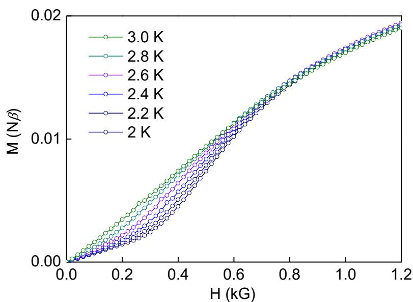
**Figure S9.** Field dependence of magnetizations for compound 1 measured at the indicated temperatures.
