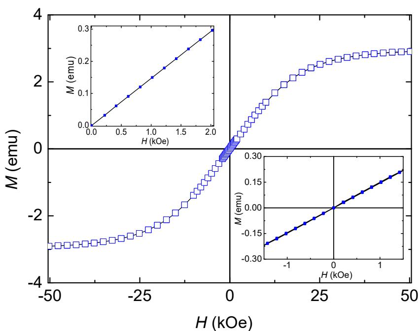
**Figure S16.** Field dependence of the magnetization of thermally decomposed compound **1** at 1.8 K. The insets give the low field range of  $M$  vs.  $H$ .
