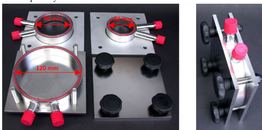
Figure S2. (Left) The components of the migration cells. Cells of three different geometrical characteristics; the cell possessing 30 mm diameter was used for the migration experiments. (Right) A typical assembly of the cell that is ready to be put into the incubating chamber.
