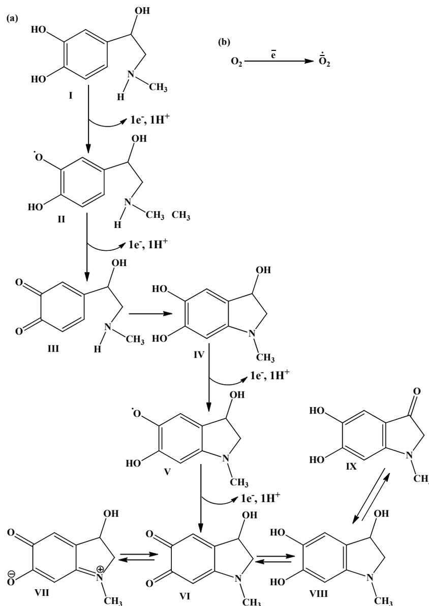
**Scheme 1.** The quinoid mechanism of adrenaline autoxidation. (a) Transformation of adrenaline I into adrenochrome VI; II–V are intermediate reaction products; possible mutual transitions of the products varying from VI (adrenochrome) to VII, VIII, and IX; (b) reaction of superoxide anion-radical formation.
