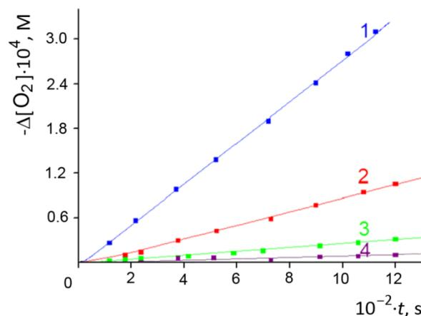
**Figure 2.** Kinetics of oxygen consumption during the oxidation of adrenaline in phosphate buffer. [AAPH] =  $4 \cdot 10^{-3}$  M; [Adr]<sub>0</sub> =  $1 \cdot 10^{-3}$  M; pH = 9.0 (1), 8.2 (2), 7.4 (3), 6.0 (4); 310 K.
