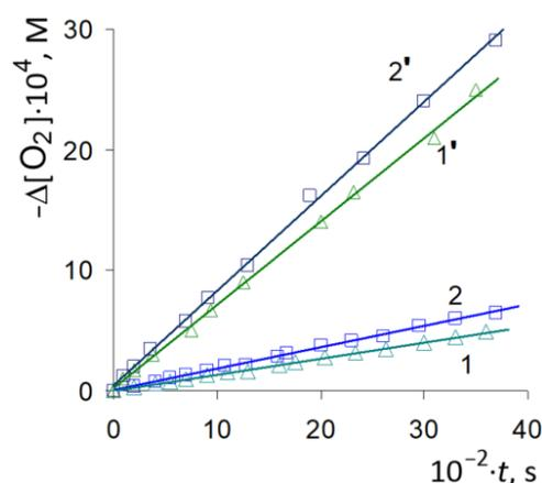
**Figure 4.** Kinetics of oxygen consumption during the oxidation of adrenaline.  $[\text{AAPH}] = 4 \cdot 10^{-3}$  M;  $[\text{Adr}]_0 = 1 \cdot 10^{-3}$  M; H = 9.0; 310 K. Carbonate buffer:  $[\text{SOD}]_0 = 100$  U/mL (1'  $\Delta$ ),  $[\text{SOD}]_0 = 0$  U/mL (2'  $\square$ ); phosphate buffer:  $[\text{SOD}]_0 = 100$  U/mL (1  $\Delta$ ),  $[\text{SOD}]_0 = 0$  U/mL (2  $\square$ ).
