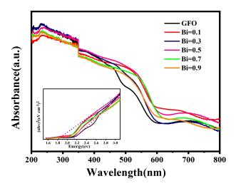
**Figure 5.** UV-vis absorption spectra of  $Gd_{1-x}Bi_xFeO_3$  nanoparticles; the inset shows the calculation of the band gaps.
