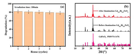
**Figure 9.** (a) Reusability of  $Gd_{0.5}Bi_{0.5}FeO_3$  nanoparticles in the degradation of MB under UV light irradiation over five cycles; (b) XRD patterns of the  $Gd_{0.5}Bi_{0.5}FeO_3$  sample before and after the photocatalytic experiment.
