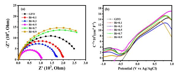
**Figure 7.** (a) Complex impedance spectra (Z' vs. Z'') and (b) Mott-Schottky plots of  $Gd_{1-x}Bi_xFeO_3$  samples at room temperature.
