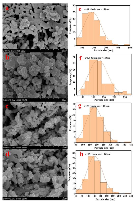
**Figure 2.** SEM image of (**a**) GFO calcined at 700  $^{\circ}$ C; (**b**) GBFO5 calcined at 700  $^{\circ}$ C; (**c**) GBFO7 calcined at 700  $^{\circ}$ C; (**d**) GBFO9 calcined at 550  $^{\circ}$ C; (**e**–**h**) statistical estimation of the particle size distribution of GFO, GBFO5, GBFO7 and GBFO9.
