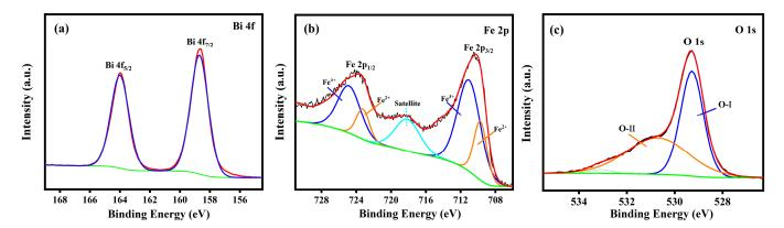
**Figure 3.** X-ray photoelectron spectroscopy (XPS) spectra of (**a**) Bi 4f, (**b**) Fe 2p and (**c**) O 1s for the  $Gd_{0.5}Bi_{0.5}FeO_3$  sample.
