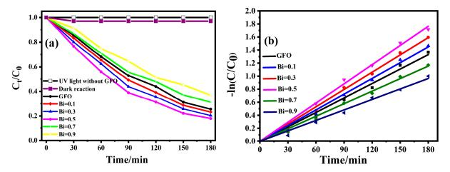
**Figure 6.** (a) Photocatalytic degradation efficiencies of MB using  $Gd_{1-x}Bi_xFeO_3$  as a catalyst; (b) pseudo-first-order kinetics fitting data for the photodegradation of MB over  $Gd_{1-x}Bi_xFeO_3$  samples.
