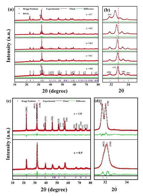
**Figure 1.** XRD patterns of (a)  $Gd_{1-x}Bi_xFeO_3$  (x = 0, 0.1, 0.3, 0.5, 0.7) annealed at 700 °C; (c)  $Gd_{1-x}Bi_xFeO_3$  (x = 0.9, 1.0) annealed at 550 °C; (b,d) enlarged view of 20 from 31° to 35°.
