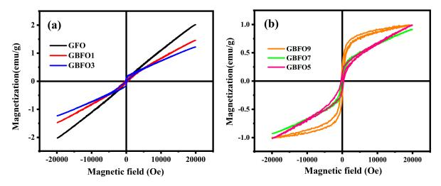
**Figure 4.** Room temperature magnetic hysteresis loops of **(a)** GFO, GBFO1 and GBFO3 samples; **(b)** GBFO5, GBFO7 and GBFO9 samples.
