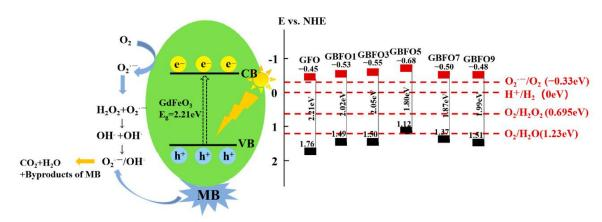
Figure 8. Schematic diagram of the band structure and proposed mechanism of the photocatalytic process.
