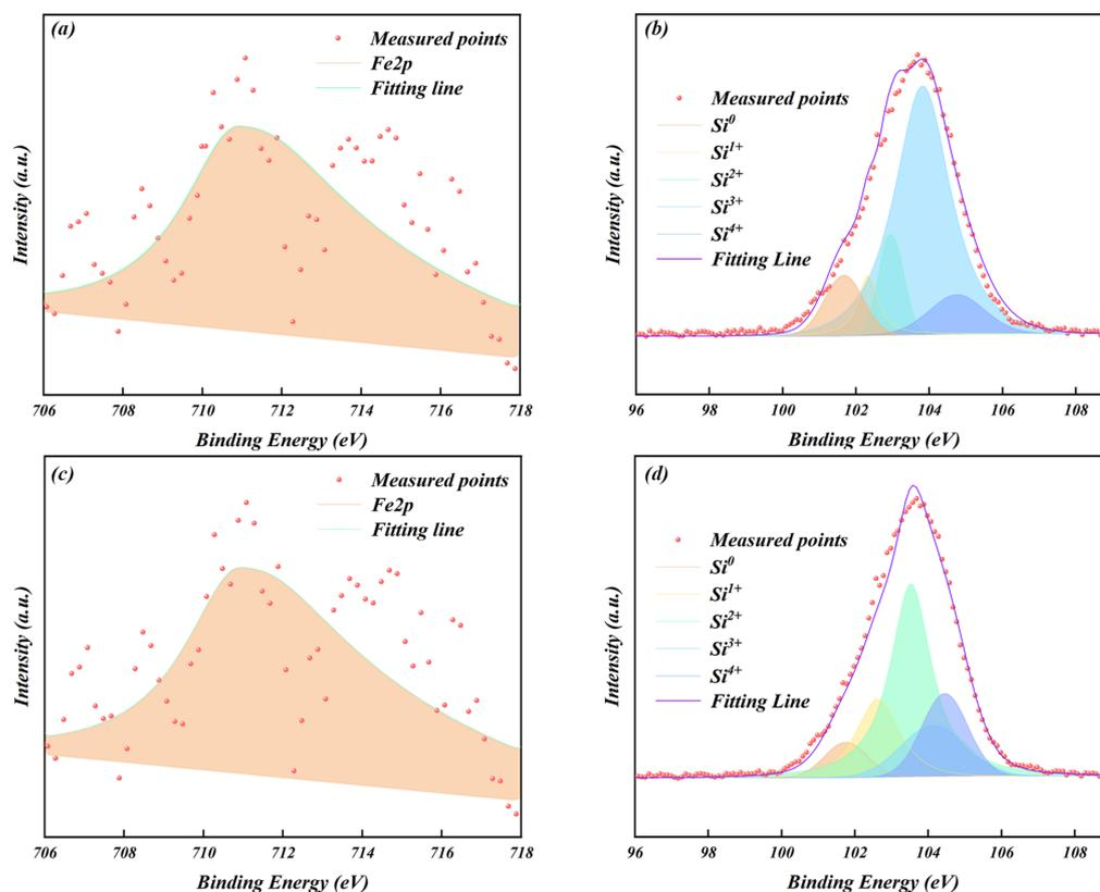
**Figure 2.** XPS results of Fe–Si–Cr composites before ((a)–Fe, (b)–Si) and after deposition ((c)–Fe, (d)–Si).
