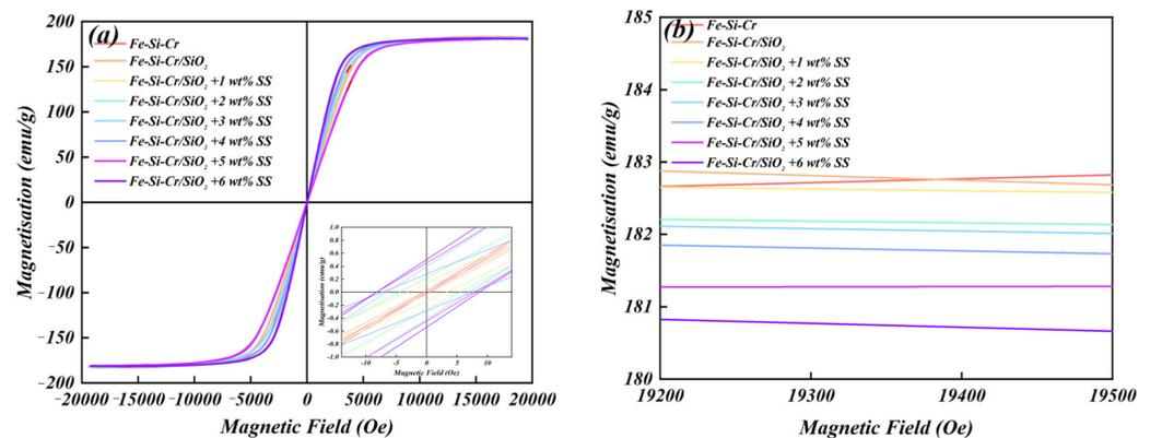
**Figure 4.** Hysteresis curves of Fe-Si-Cr-based SMCs showing changes in saturation magnetization (a) and coercivity (b).
