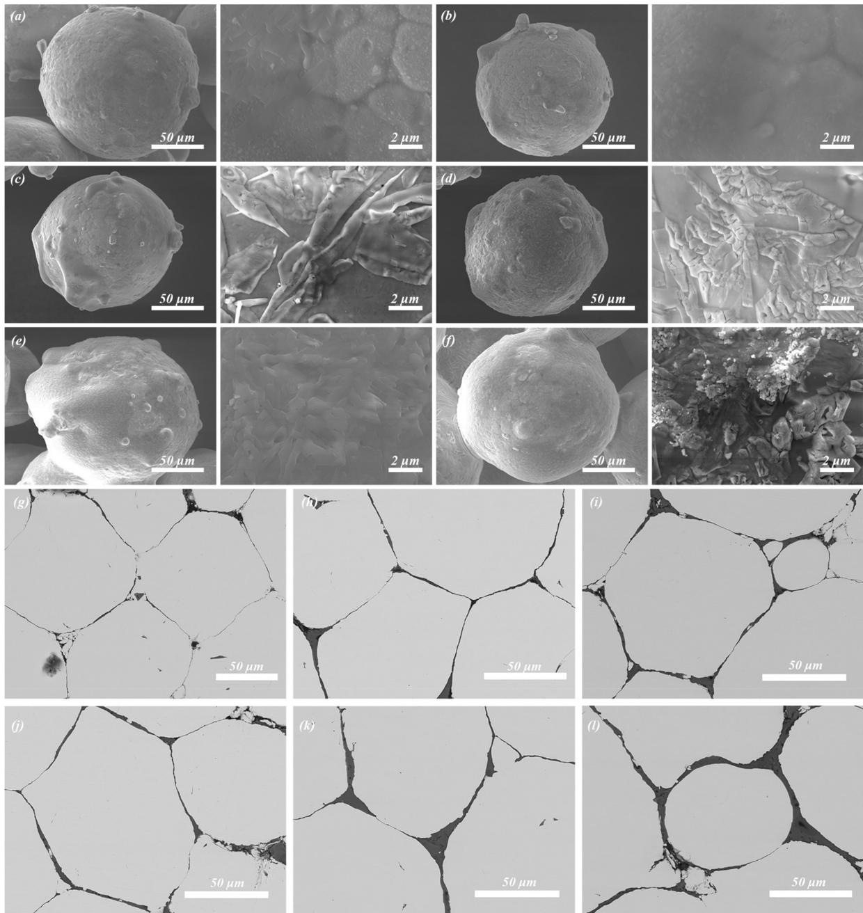
**Figure 3.** SEM images of the Fe-Si-Cr composites before (a,g) and after deposition (b-f,h-l).
