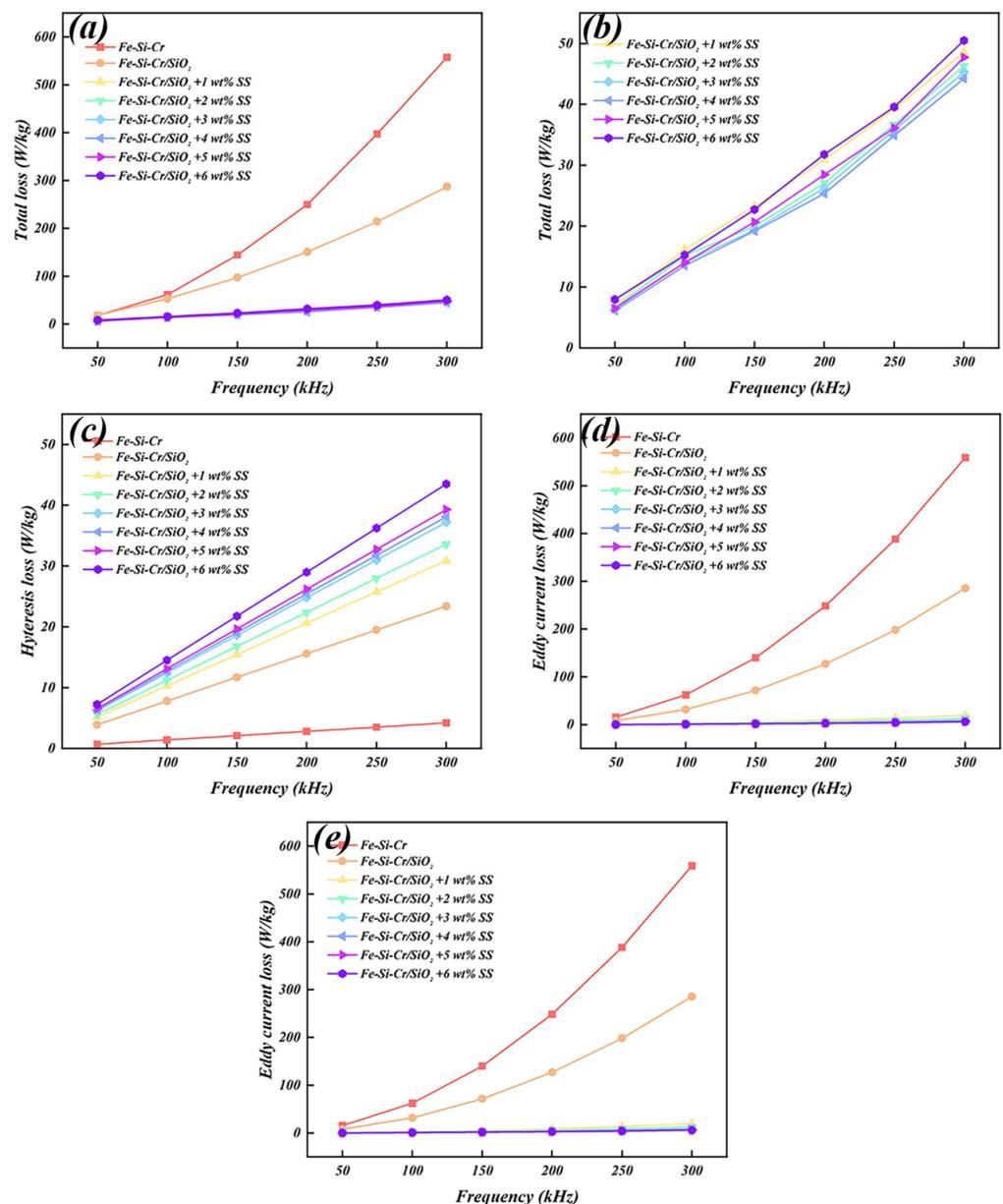
**Figure 6.** Total loss (a,b), hysteresis loss (c), and dynamic loss (d,e) of SMCs with various insulating layers measured at 10 mT and 50–300 kHz.
