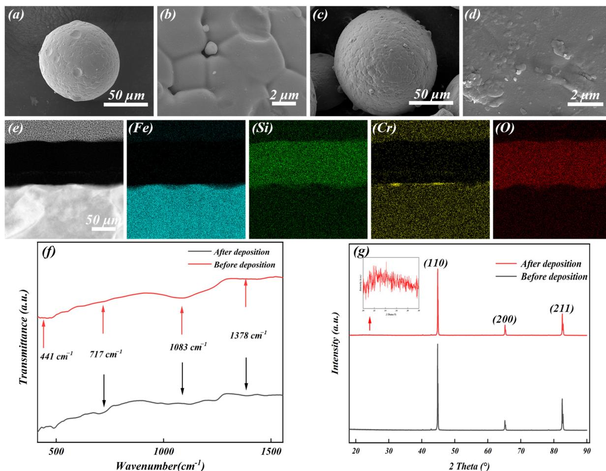
**Figure 1.** SEM images of Fe-Si-Cr powders prior to (a,b) and after deposition (c,d); EDS spectra (e), FTIR spectra (f), and XRD patterns (g).
