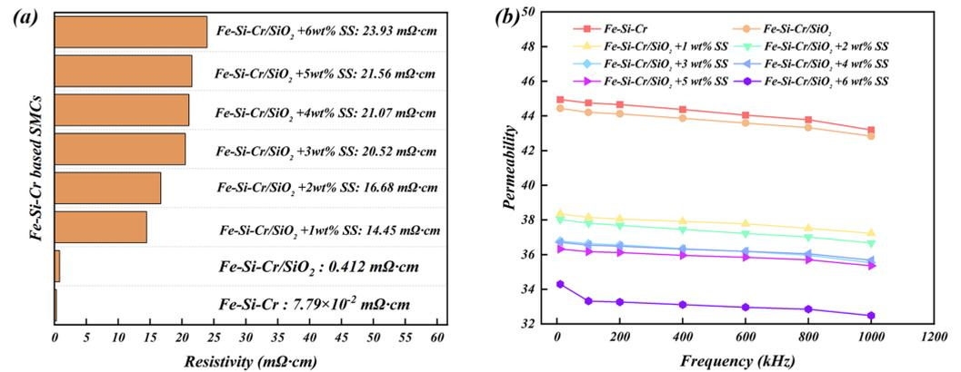
Figure 5. Trends in the resistivity (a) and permeability (b) of Fe-Si-Cr-based SMCs.
