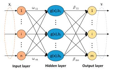
Figure 6. The network structure of ELM.
