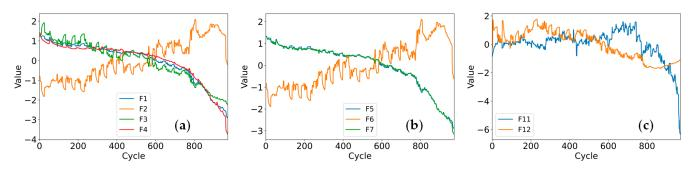
Figure 4. Standardized health indicators of CS2\_37: (a) Type1; (b) Type2; (c) Type4.
