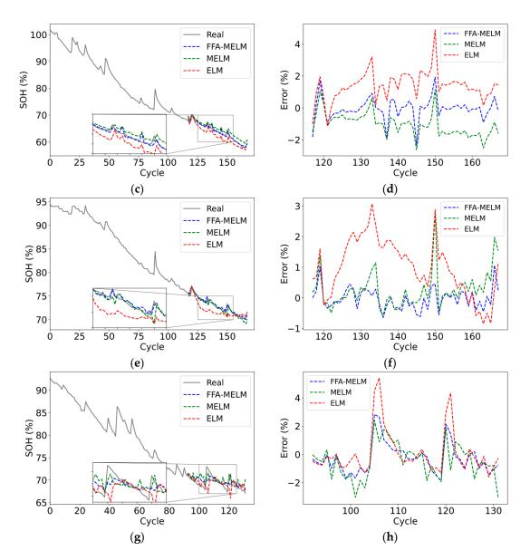
**Figure 10.** SOH estimation experiments of different methods under mild operating conditions. Estimation results: (**a**) B05; (**c**) B06; (**e**) B07; (**g**) B18. The estimation error of the test data: (**b**) B05; (**d**) B06; (**f**) B07; (**h**) B18.
