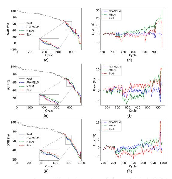
**Figure 13.** SOH estimation experiments of different methods for CALCE. Estimation results: (a) CS2\_35; (c) CS2\_36; (e) CS2\_37; (g) CS2\_38. Estimation error of the test data: (b) CS2\_35; (d) CS2\_36; (f) CS2\_37; (h) CS2\_38.
