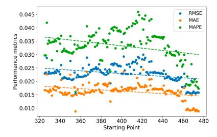
Figure 15. Performance metrics of different starting points ranging from 325 to 475 cycles for CS2\_35.
