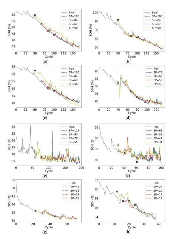
**Figure 12.** SOH estimation results at different starting test points: (**a**) B05; (**b**) B06; (**c**) B07; (**d**) B18; (**e**) B34; (**f**) B55; (**g**) B45; (**h**) B31.
