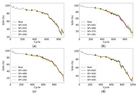
**Figure 14.** SOH estimation results at different starting test points for CALCE: (**a**) CS2\_35; (**b**) CS2\_36; (**c**) CS2\_37; (**d**) CS2\_38.
