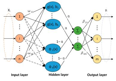
Figure 7. The network structure of MELM.
