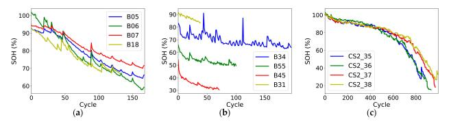
**Figure 1.** Battery capacity decline curve: (**a**) NASA mild operating conditions; (**b**) NASA complex operating conditions; (**c**) CALCE.
