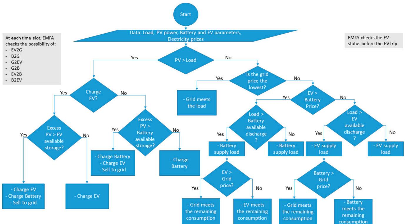
Figure 3. The EFMS algorithm.
