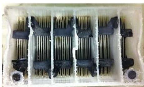
Figure 1. A 12 V lead acid battery with its lid sawn off to show the six compartments containing five negative and four positive electrode sets each. Lead current collectors are connected to each electrode and the positive connections connected together, as are the negative electrodes. The connection is maintained along the six cell in series, and terminate at two external leads.
