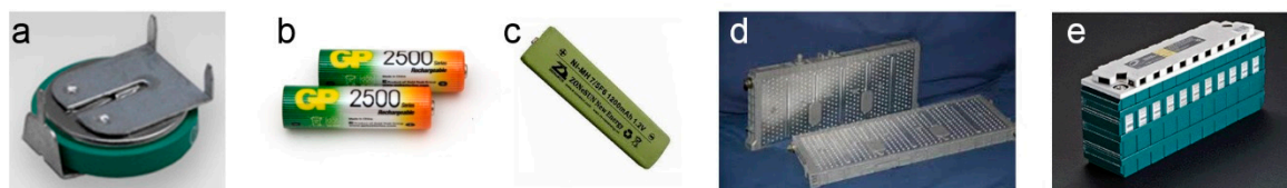
Figure 1. Nickel/metal hydride (Ni/MH) batteries in (a) a coin cell, (b) a cylindrical cell, (c) a stick cell (small prismatic), (d) an EV cell (large prismatic), and (e) an hybrid electric vehicles (HEV) cell (large prismatic).
