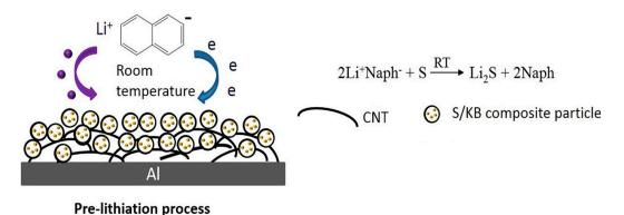
**Figure 18.** Chemical pre-lithiation process of a sulphur composite positive electrode. The Li-organic complex solution served as lithium source for this pre-lithiation technique. Reproduced with permission from [196] Copyright 2017, Elsevier.
