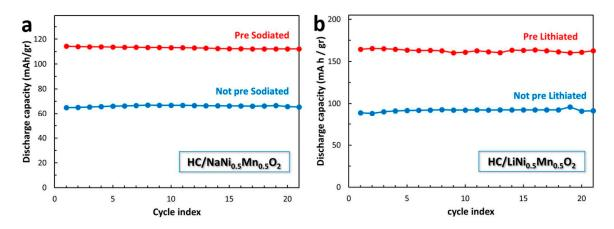
**Figure 2.** Effect of negative electrode pre-treatment on the discharge capacity of sodium and lithium ion cells. (a) Hard carbon(HC)/NaNi<sub>0.5</sub>Mn<sub>0.5</sub>O<sub>2</sub> (b) Hard carbon/LiNi<sub>0.5</sub>Mn<sub>0.5</sub>O<sub>2</sub>. Reproduced with permission from [34] Copyright 2016, American Chemical Society.
