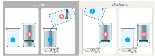
**Figure 1.** Schematic illustration of (**a**) active lithium loss (ALL) in the 1st charge/discharge cycle in a lithium ion cell and concepts for reducing the active lithium loss by pre-lithiation, i.e., (**b**) by pre-lithiation of the negative electrode (-) or (**c**) by pre-lithiation with help of the positive electrode (+).
