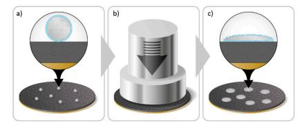
**Figure 9.** Schematic illustration of the pressure induced activation process of stabilized Li metal powder (SLMP): (a) Application of SLMP on electrode surface; (b) Pressure induced activation; (c) Electrode surface after activation.
