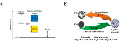
**Figure 12.** (a) Schematic drawing of the required working potential of the pre-lithiation additive. Reproduced with permission from [114] Copyright 2017, Springer Nature. (b) Synthesis of the  $Li_2S/Co$ . additive and the release of the  $Li^+$  during the initial cycle. Reproduced with permission from [115] Copyright 2017, Wiley-VCH.
