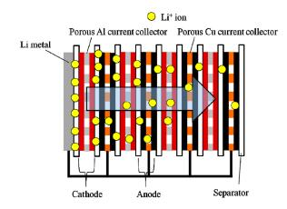
**Figure 16.** A schematic illustration of the pre-lithiation system, which is commercially used for the fabrication of LICs. Laminated carbon anodes with porous current collectors are pre-lithiated by using an auxiliary Li metal electrode. Reproduced with permission from [167] Copyright 2017, Electrochemical Society, Inc.
