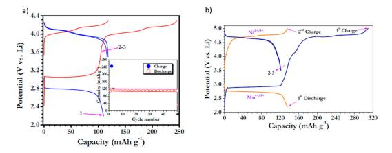
**Figure 14.** De-lithiation and lithiation of o-LMO (**a**) and *o*-LNMO (**b**) in a Li metal cell. Firstly, pristine LMO and LNMO are over-lithiated by controlling the cut-off potentials. Subsequently the *o*-LMO and *o*-LNMO are cycled in the potential range the tetrahedral site. Reproduced with permission from (**a**) [131] Copyright 2017, Elsevier. (**b**) [136] Copyright 2017, Elsevier.
