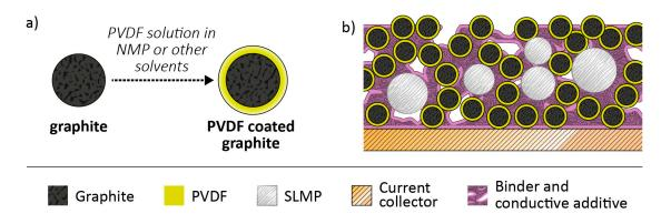
**Figure 10.** (a) Schematic model of PVdF coated graphite particles. (b) Schematic model for a SLMP incorporated graphite negative electrode, based on a SBR-PVDF dual binder approach. Adapted with permission from [76] Copyright 2013, Royal Society of Chemistry.
