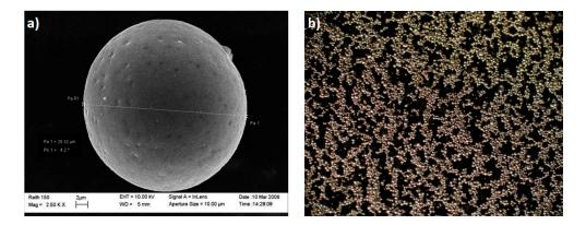
**Figure 8.** (a) SEM image of a single spherical SLMP particle; (b) microscopic image of sprayed SLMP on a pre-fabricated negative electrode sheet. Reproduced with permission from [71] Copyright 2011, Elsevier.
