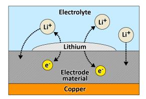
Figure 6. Schematic illustration of the pre-lithiation process by direct contact to Li metal.
