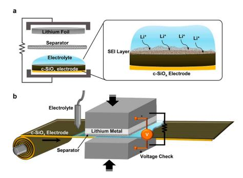
**Figure 3.** (a) Graphical illustration of the pre-lithiation process of a c-SiO<sub>x</sub> negative electrode and (b) its scalable roll-to-roll process scheme. Reproduced with permission from [30] Copyright 2016, American Chemical Society.
