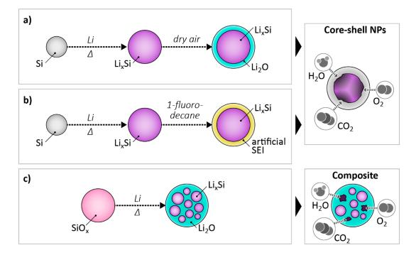
Figure 11. Schematic diagram comparing different approaches in order to produce a pre-lithiation additive for the negative electrode. (a) Lithium oxide protected lithium silicide core-shell nanoparticles.(b) Artificial SEI protected lithium silicide core-shell nanoparticles. (c) Lithium silicide/lithium oxide composite.
