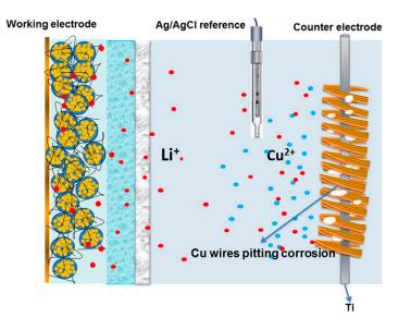
**Figure 5.** Principle of pre-lithiation of a Si-based working electrode by using an electrolytic cell with a copper pitting corrosion type anodic half-cell in aqueous electrolyte ( $0.5M Li_2SO_4$ ) and a LIB type cathodic half-cell in gel polymer electrolyte (GPE) soaked in 1M LiPF<sub>6</sub> in ethylene carbonate (EC)/diethyl carbonate (DEC) electrolyte (3:7 v/v). Reproduced with permission from [58] Copyright 2015, Wiley-VCH.
