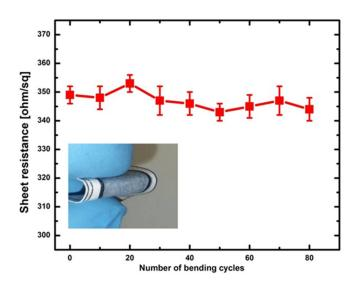
Figure 4. Sheet resistance of the anodic chamber vs. the number of bending cycles.
