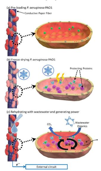
**Figure 5.** Schematic illustration of bacteria storage, their rehydration with wastewater, and their power generation. (**a**) Pre-loading bacterial cells in the anodic reservoir, (**b**) freeze-drying the device with the cells, and (**c**) rehydrating the cells for on-demand power generation.
