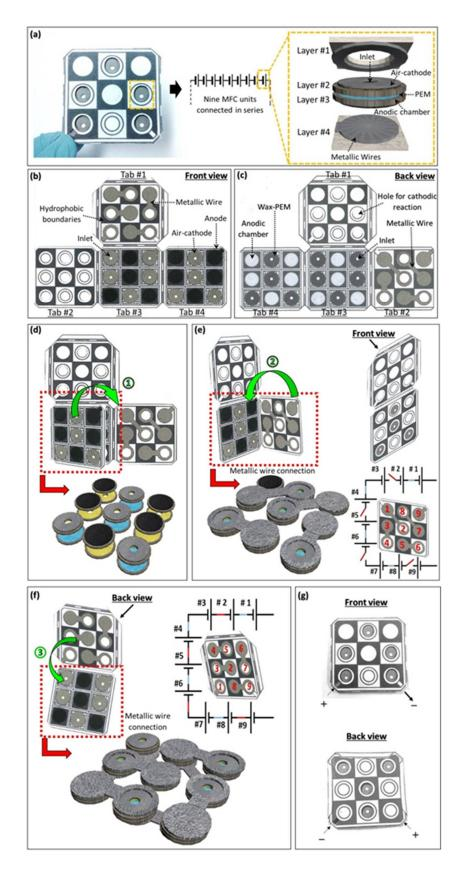
**Figure 1.** (a) An origami paper-based biobattery stack and schematic diagram of a cross-section of the single unit; (b) Front and (c) back view of the two-dimensional (2-D) sheet of paper before folding; (d–f) Folding processes for the three-dimensional (3-D) battery stack and its metallic wire configuration; (g) Front and back view of the folded battery stack.
