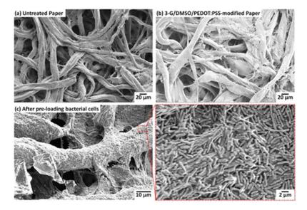
**Figure 3.** SEM (Scanning electron microscope) images of the anodic chamber. (**a**) Non-treated paper and 3-G/DMSO/PEDOT:PSS-treated paper (**b**) without and (**c**) with bacterial cells. 3-G: 3-glycidoxypropy-trimethoxysilane; DMSO: dimethyl sulfoxide; PEDOT:PSS: poly(3,4-ethylenedioxythiophene):poly(styrene sulfonate).
