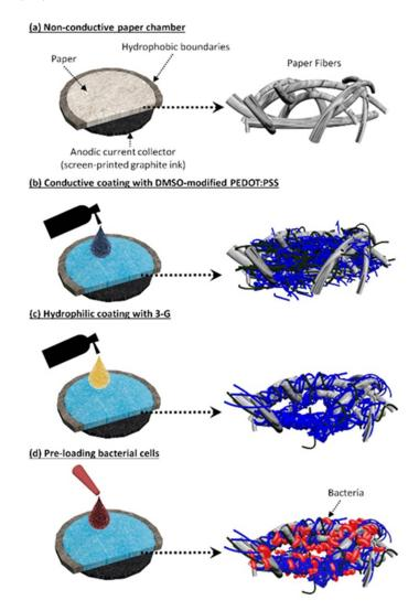
**Figure 2.** Schematic illustration of the fabrication steps for conductive and hydrophilic anodic chambers. (a) Defining Hydrophobic boundaries, (b) Conductive engineering the anodic reservoir, (c) Hydrophilic coating of the reservoir, and (d) pre-loading exoelectrogens.
