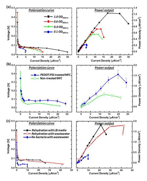
**Figure 7.** Polarization curves and power outputs measured from the single MFCs (**a**) with different concentrations of non-freeze-dried bacterial cells; (**b**) with 1.0 OD600 culture of non-freeze-dried cells in the anodic chamber with or without PEDOT:PSS treatment; and (**c**) with rehydrated freeze-dried cells (1.0 OD600 culture) in a different liquid. A control without bacterial cells was also prepared for comparison.
