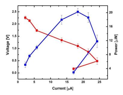
Figure 8. Polarization curves and output powers measured from the nine-MFC stack with wastewater activation liquid.
