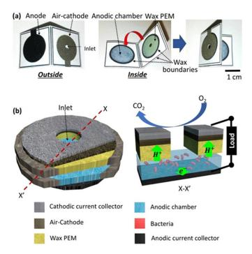
Figure 6. (a) Photos and (b) schematics of the single microbial fuel cell (MFC) unit.
