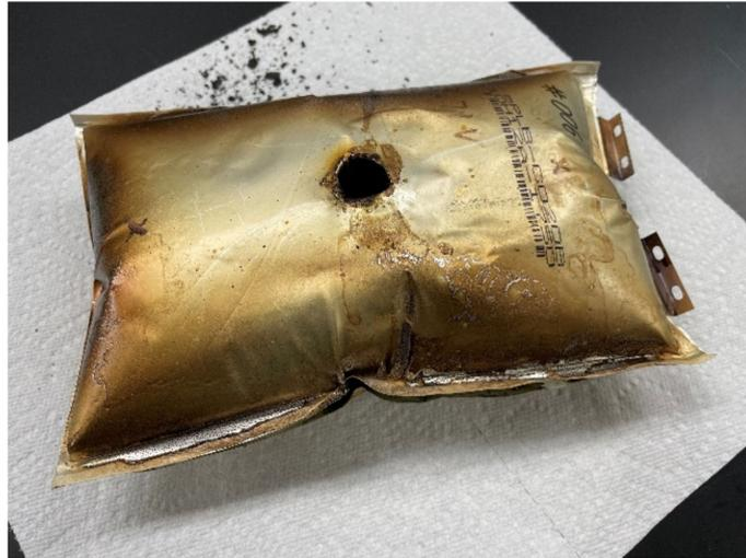
**Figure 3.** Battery cell after the combustion during the penetration test.
