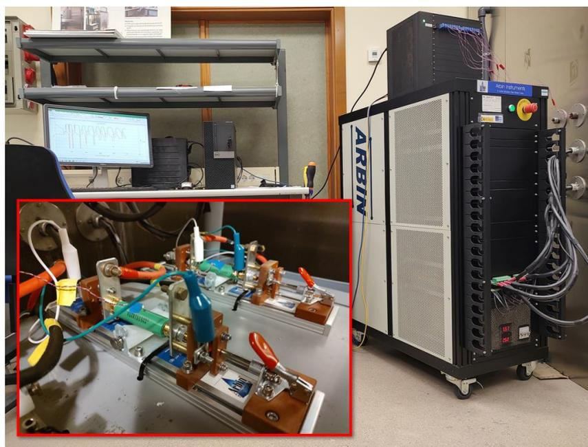
**Figure 1.** Photographs of the test equipment and some cells under test.
