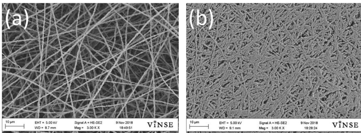
**Figure 2.** SEM images of (a) raw electrospun Si/PAA (40 wt.% PAA) fiber mat, and (b) final electrode obtained after fiber welding and mat densification. Magnification 3000 $\times$ .
