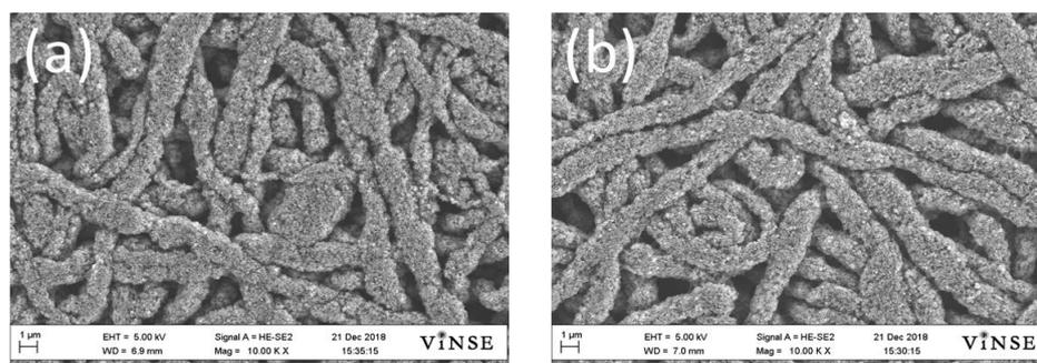
**Figure 7.** SEM images of compacted electrospun single fiber Si/PAA-C anodes with (a) lower carbon content (6 wt.%), and with (b) higher carbon content (12 wt.%). Magnification 10,000 $\times$ .
