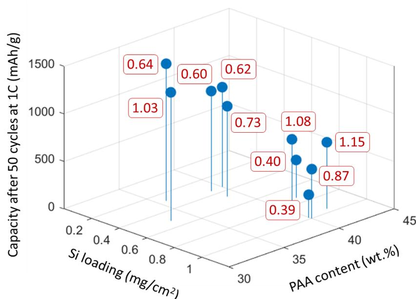
**Figure 4.** Summary comparison of discharge capacities of fiber mat anode coin cells after 50 cycles at 1C, where the anode mats contained Si and PAA only (no carbon). The box labels next to the data points show areal discharge capacities in mAh/cm<sup>2</sup>.
