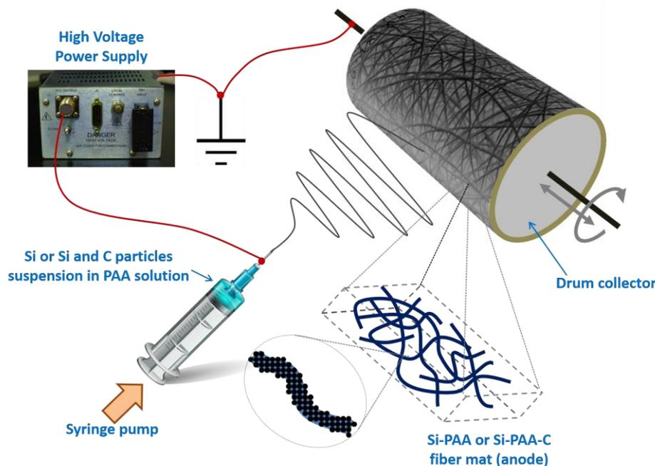
**Figure 1.** Schematic of the anode mat fabrication process by electrospinning of Si/PAA or Si/PAA/C suspensions.
