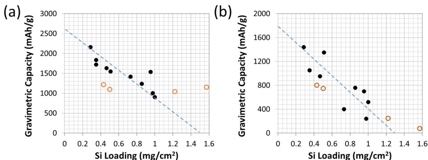
**Figure 5.** The effect of Si areal loading on gravimetric capacity for electrospun single fiber Si/PAA anodes (full circles) and slurry-cast Si/PAA anodes (open circles) after 5 cycles at 0.1C (a) and an additional 50 cycles at 1C rate. (b) Electrospun anodes contained 33–42 wt.% PAA and slurry-cast anodes contained 40 wt.% PAA.
