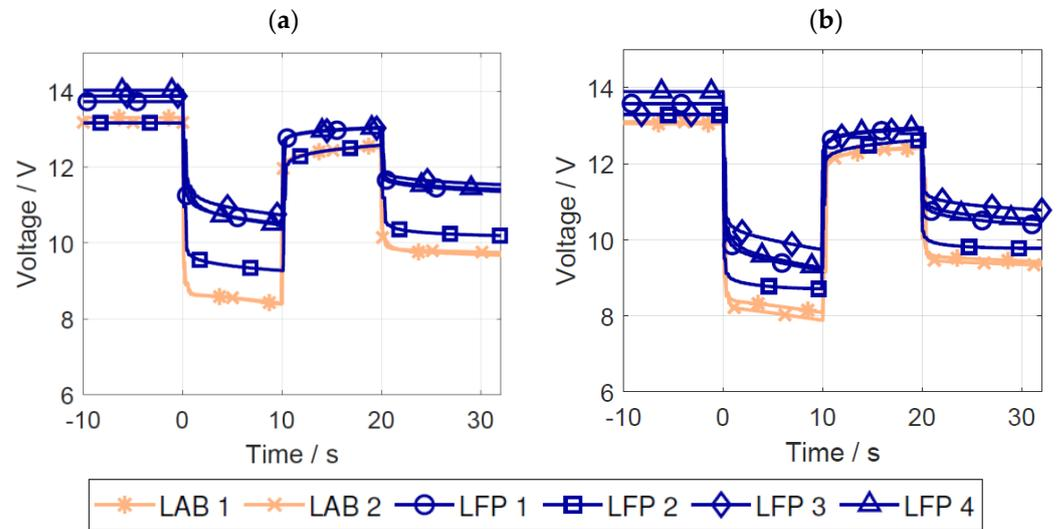
Figure 3. Cold-cranking test (a) at  $0\text{ }^{\circ}\text{C}$  and (b) at  $-10\text{ }^{\circ}\text{C}$ .
