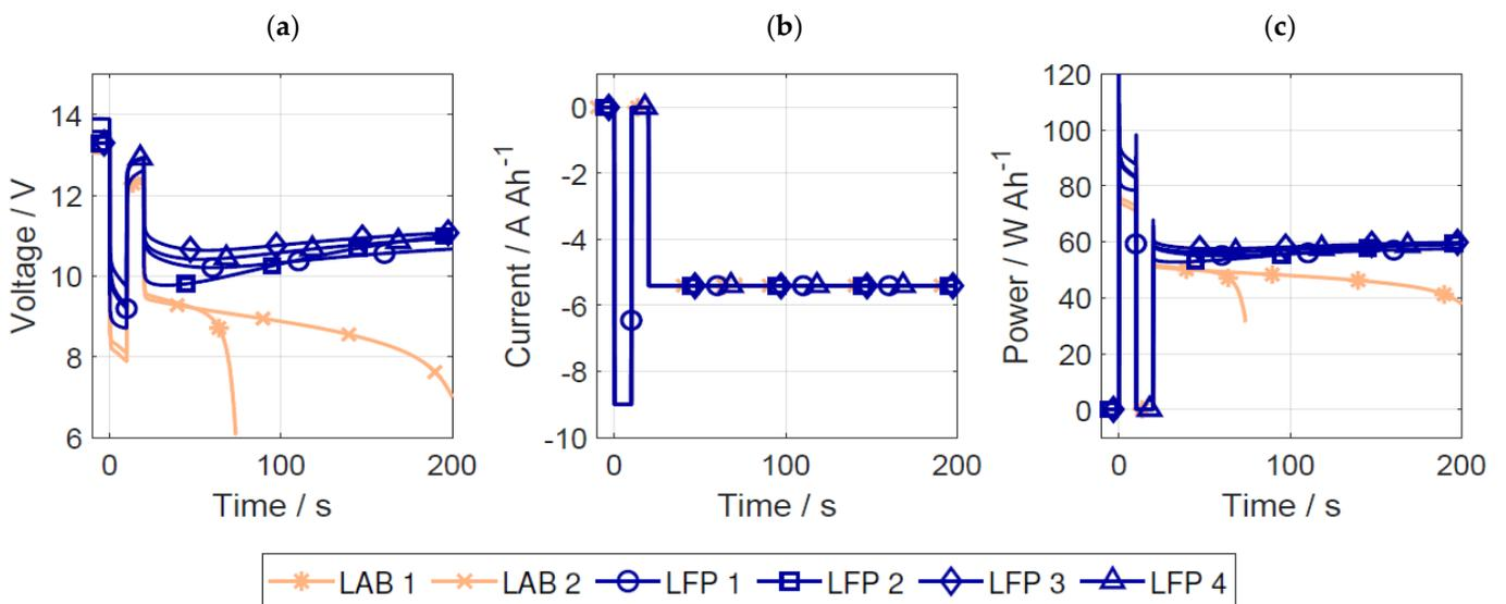
**Figure A2.** Complete cold-cranking test at -10 °C: (a) voltage, (b) current, and (c) power.
