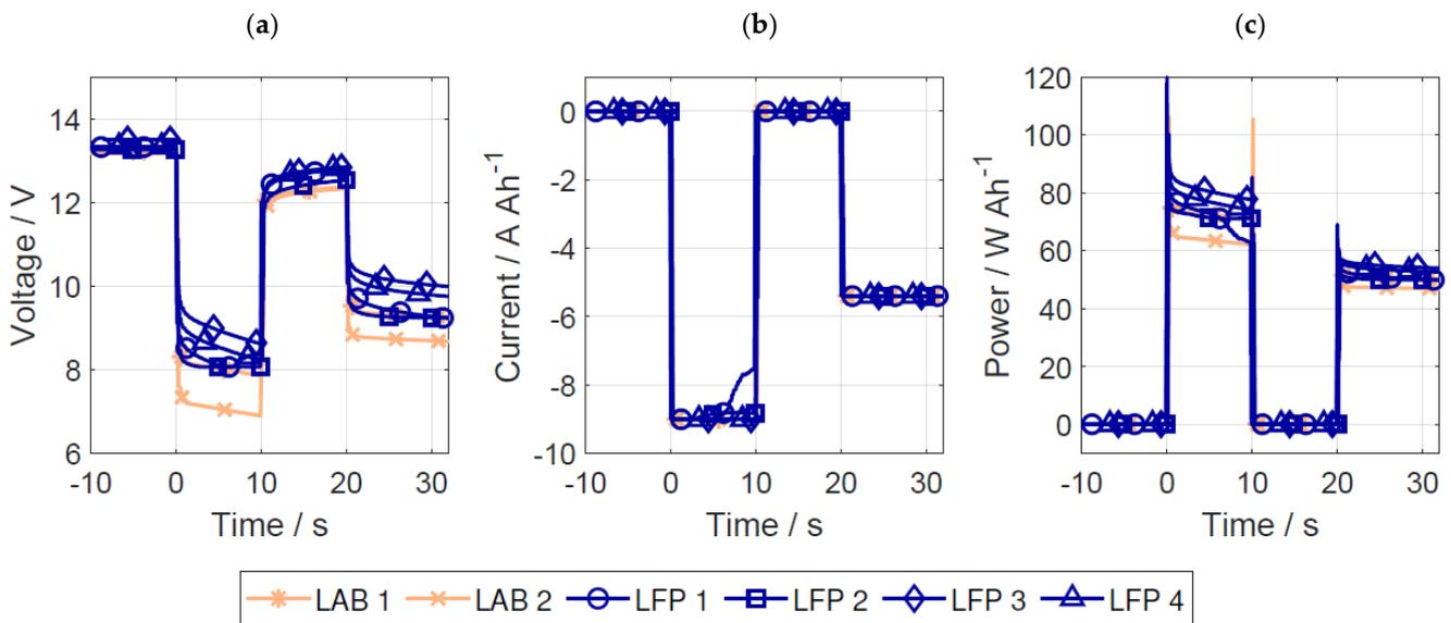
Figure 4. First pulse of the cold-cranking test at  $-18\text{ }^{\circ}\text{C}$ : (a) voltage, (b) current, and (c) power.
