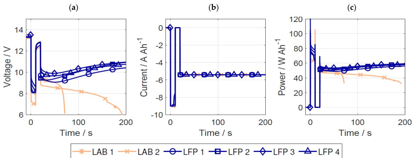
Figure A3. Complete cold-cranking test at  $-18\text{ }^{\circ}\text{C}$ : (a) voltage, (b) current, and (c) power.
