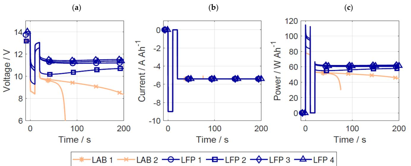
**Figure A1.** Complete cold-cranking test at 0 °C: (a) voltage, (b) current, and (c) power.
