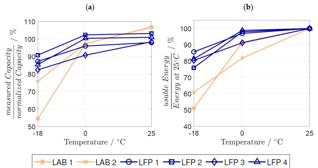
**Figure 2.** C<sub>20</sub> capacity test (a) measured capacity and (b) useable energy.
