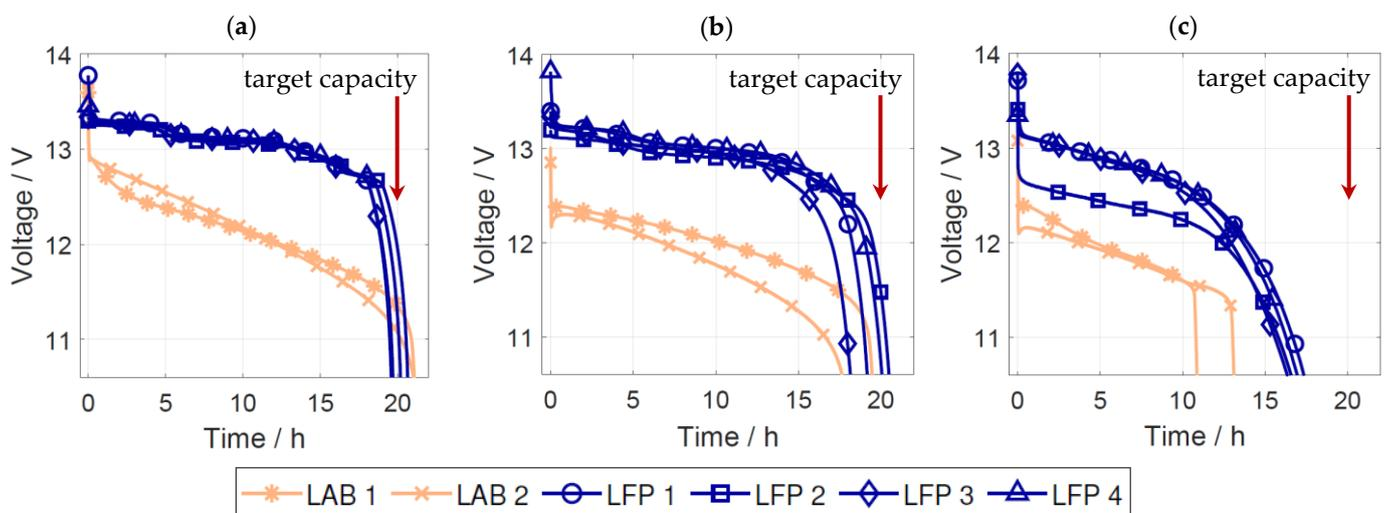
**Figure 1.**  $C_{20}$  capacity at (a)  $25^\circ\text{C}$ , (b)  $0^\circ\text{C}$ , and (c)  $-18^\circ\text{C}$ .
