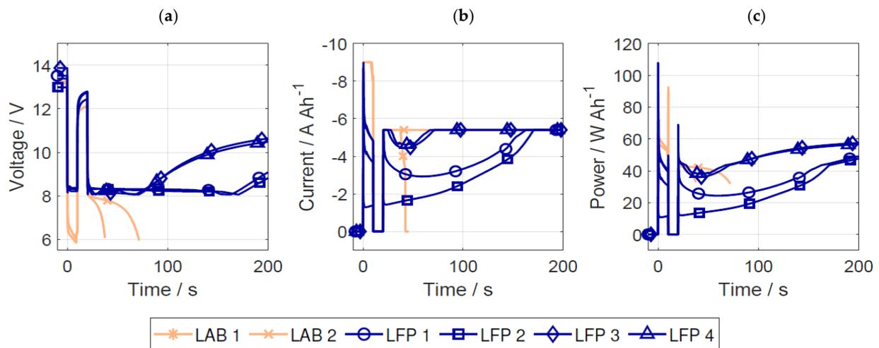
**Figure 10.** Complete cold-cranking test at  $-30\text{ }^{\circ}\text{C}$ : (a) voltage, (b) current, and (c) power.
