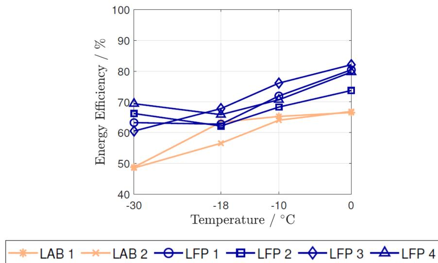
Figure 8. Energy efficiency during first pulse of cold-cranking test.
