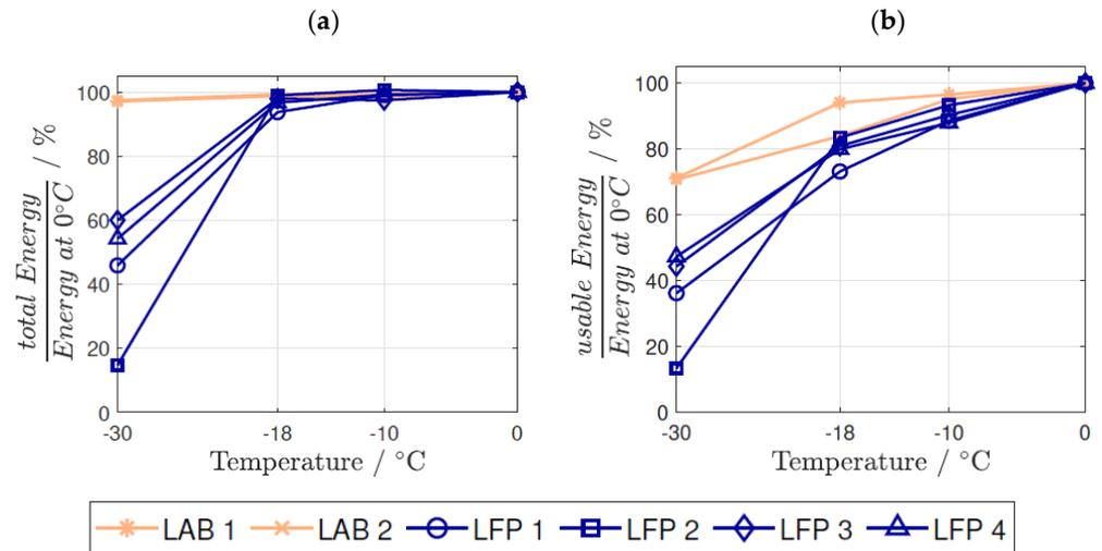
Figure 7. During the first pulse of cold-cranking test (a) total energy and (b) usable energy.
