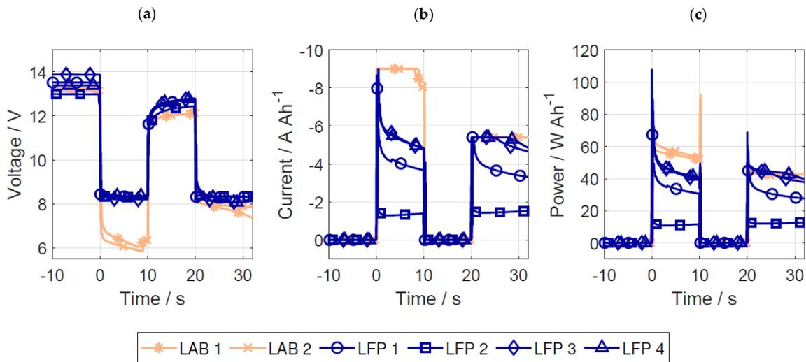
**Figure 5.** First pulse of the cold-cranking test at  $-30\text{ }^{\circ}\text{C}$ : (a) voltage, (b) current, and (c) power.
