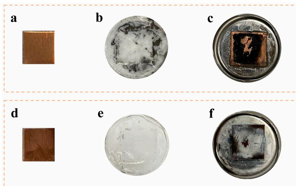
**Figure 4.** The optical images of pristine Cu foil (a), Au@CuPPA (d), and corresponding separators (b,e) and electrodes (c,f) after 30 cycles.
