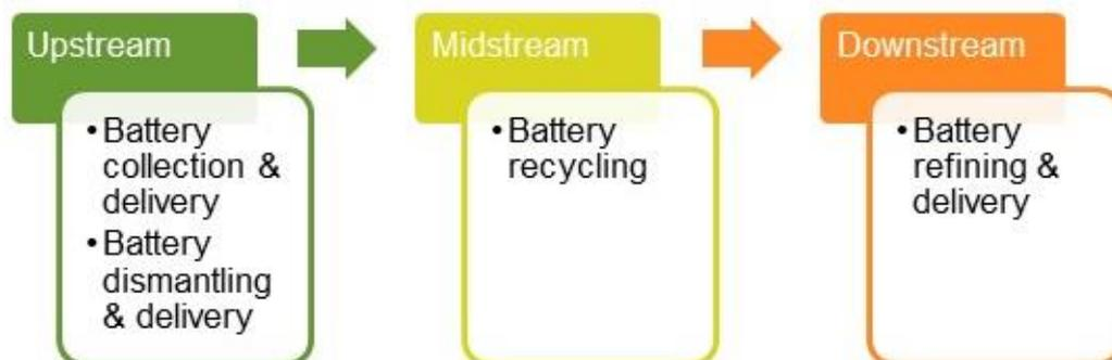
**Figure 1.** High-level description of the three recycling supply chain stages for the battery cathode active materials.
