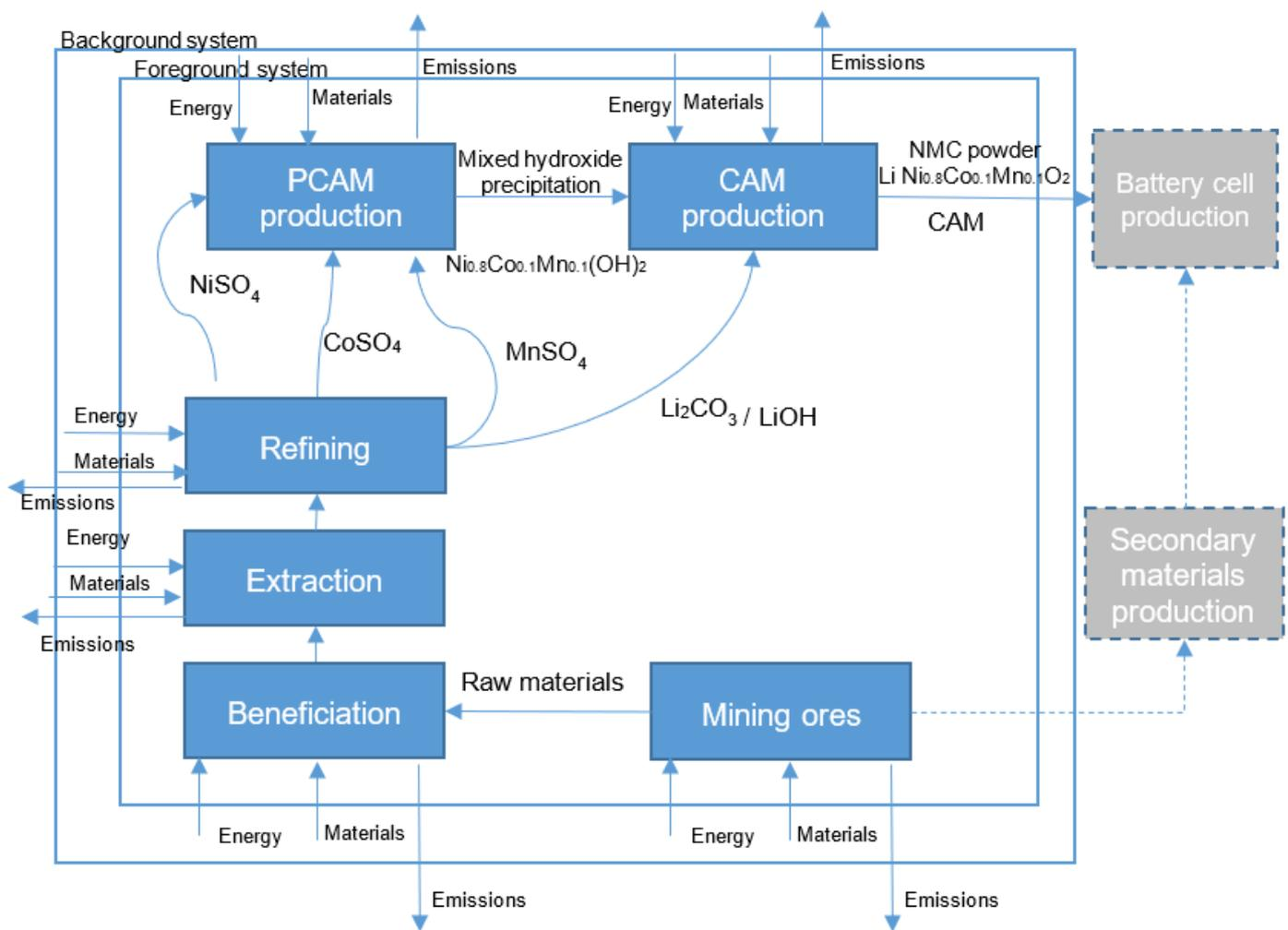
**Figure 4.** System boundary and process flow diagram of cathode active material production from virgin materials: Li, Ni, Mn, and Co.
