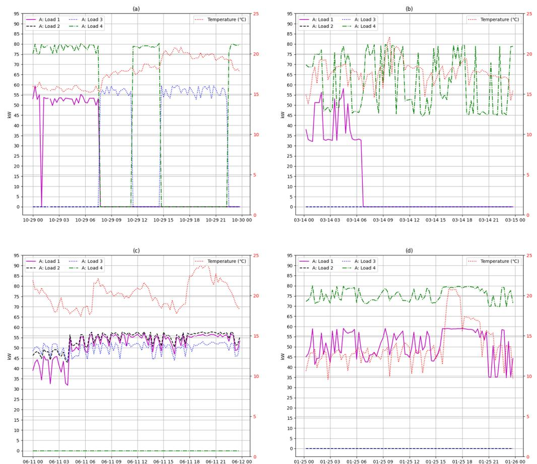
**Figure 8.** Patterns of main loads and temperature variations in the bio-manufacturing. (a) Load and temperature patterns in the fall; (b) load and temperature patterns in the spring; (c) load and temperature patterns in the summer; (d) load and temperature patterns in the winter.
