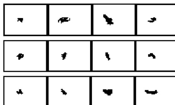
**Figure 6.** Images of particles larger than 100 µm taken by built-in camera in Qicpic.
