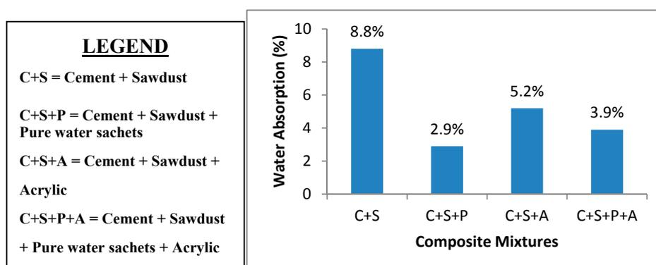
**Figure 6.** Water absorption of the composites.
