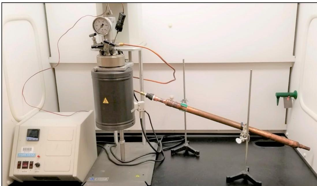
**Figure 3.** Parr reactor and Parr 4843 controller setup for slow-pyrolysis experiments.
