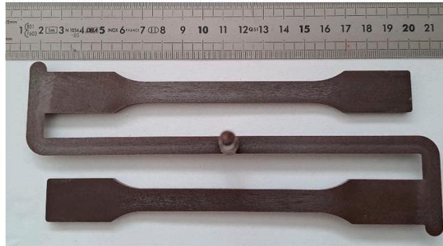
**Figure 2.** Specimens derived by injection molding (reported composition is of PLA\_CSS).
