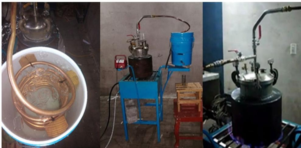
**Figure 2.** Equipment and reactor for pyrolysis.
