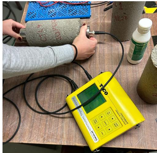
**Figure 10.** UPV test on a concrete specimen.
