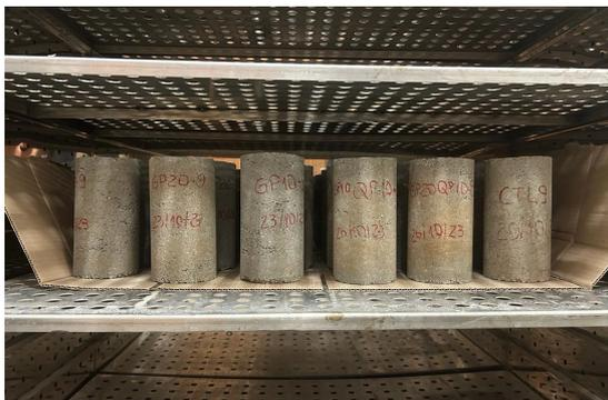
**(a)** Concrete specimens in the oven
