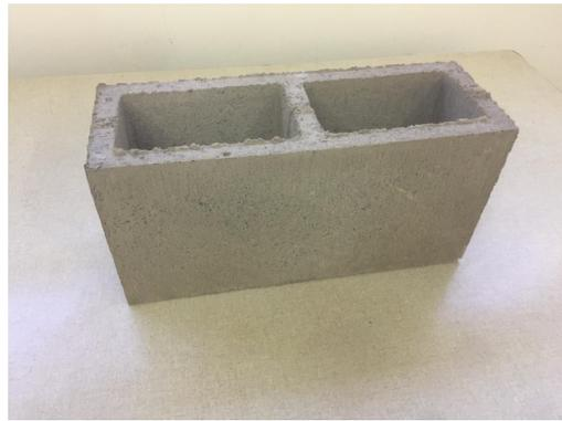
**Figure 1.** Non-structural concrete masonry block.
