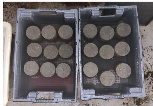
**(b)** Concrete specimens in water immersion
