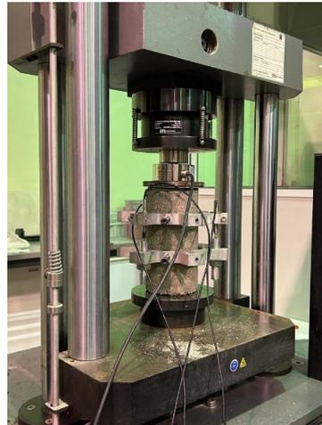
**Figure 8.** Modulus of elasticity test on a concrete specimen.
