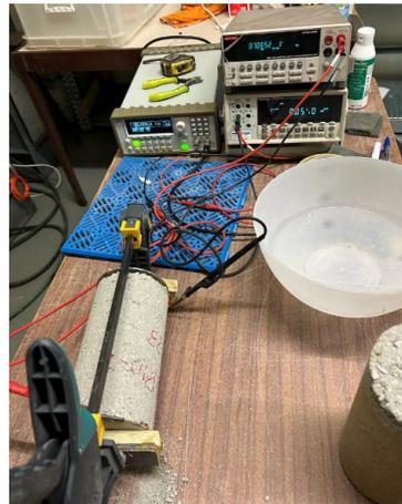
**Figure 11.** Electrical resistivity test on a concrete specimen.
