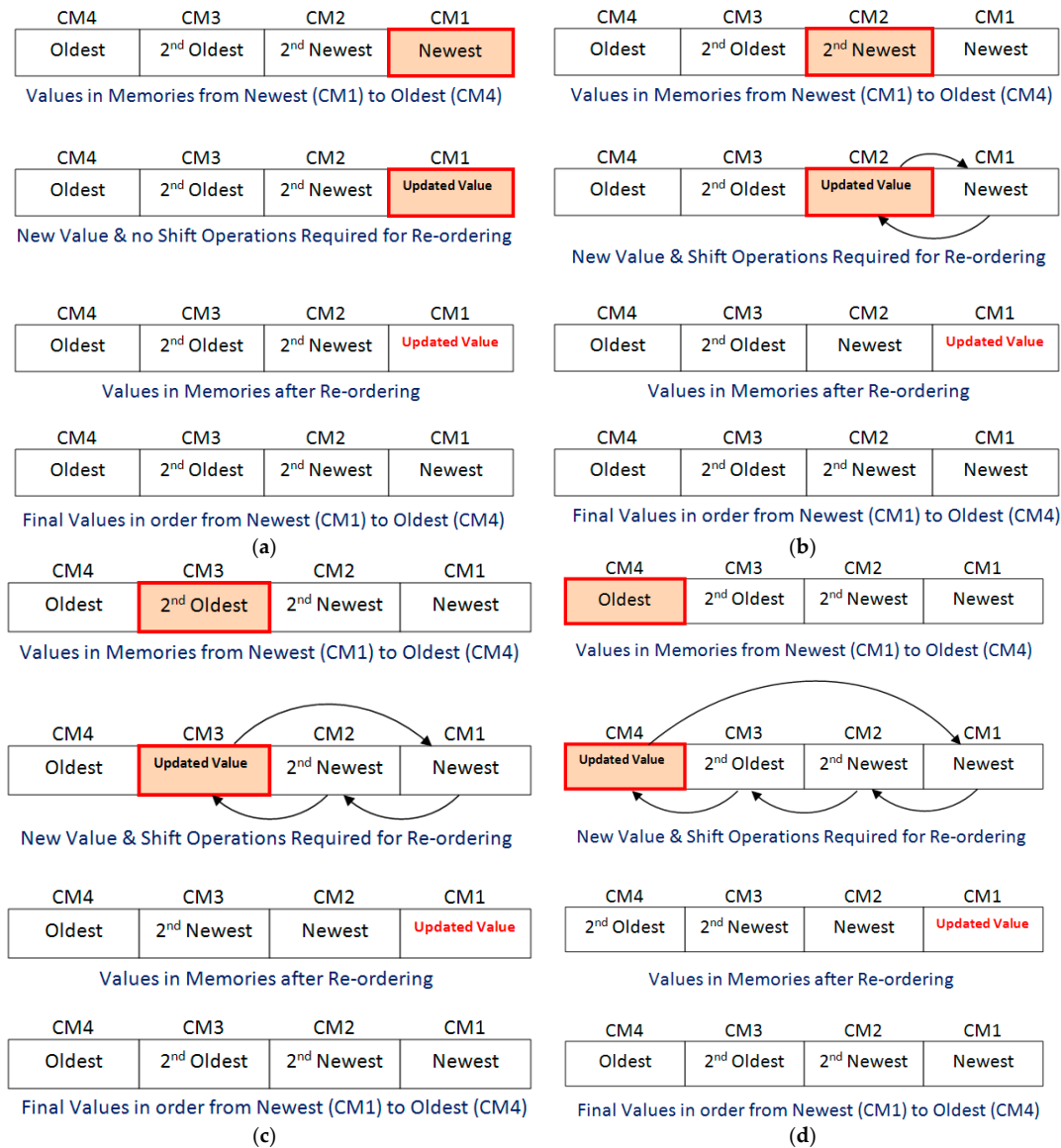
Figure 2. Cluster updating process: (a) first case; (b) second case; (c) third case; (d) fourth case.
