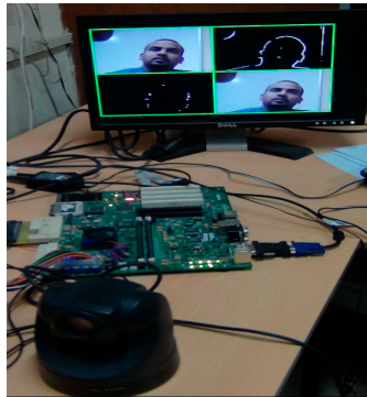
Figure 21. Complete motion detection system setup.
