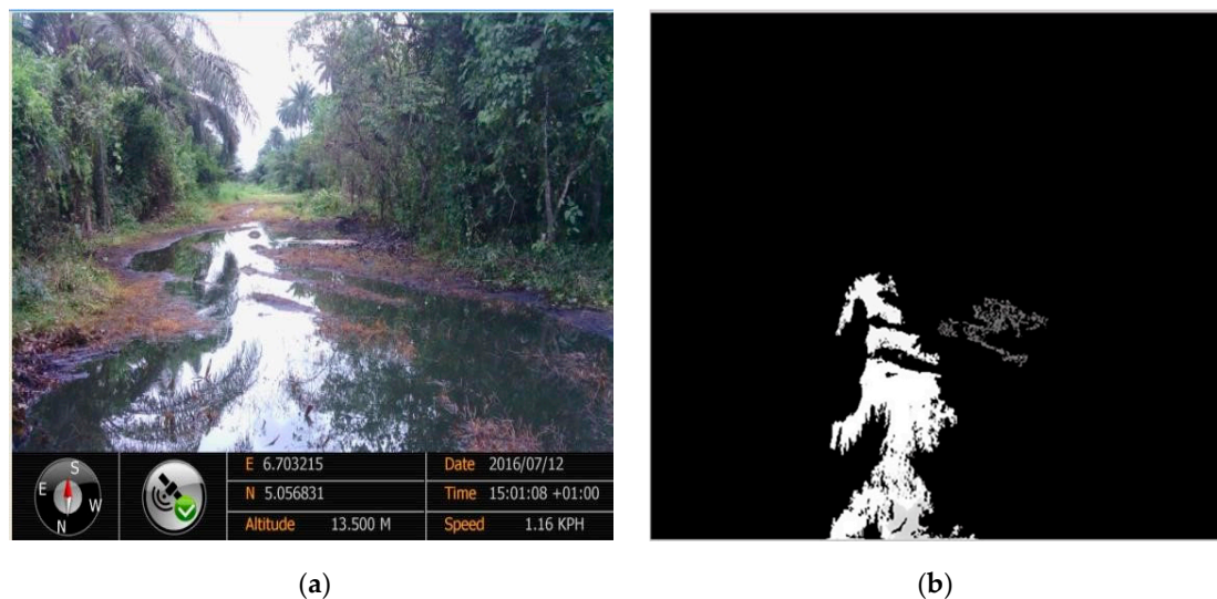
Figure 8. (a) Sample Image OS9; (b) Detected crude oil spill from OS9.
