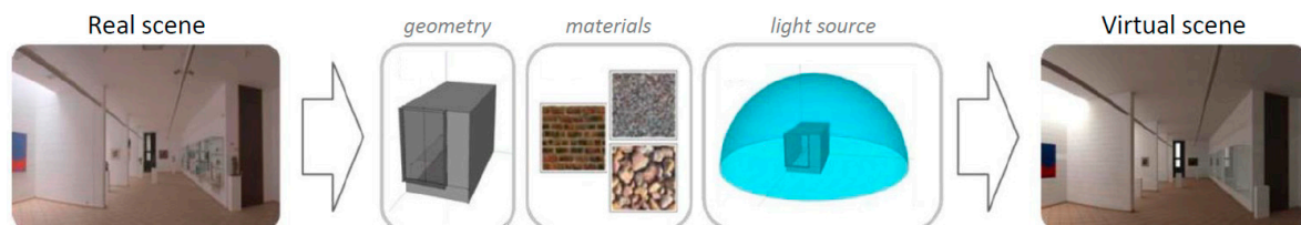
Figure 5. The virtualization of a real scene with Radiance requires describing the geometry, the materials, and the light source.
