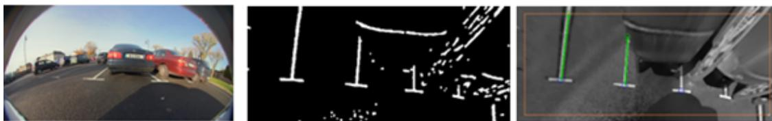
**Figure 4.** Example of parking slot marking recognition.
