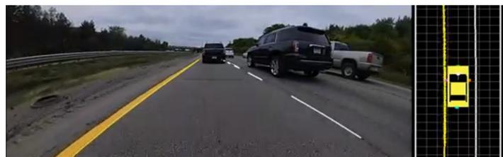
**Figure 3.** Example of road marking detection.
