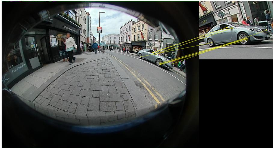
Figure 8. Illustration of ORB based feature matching.
