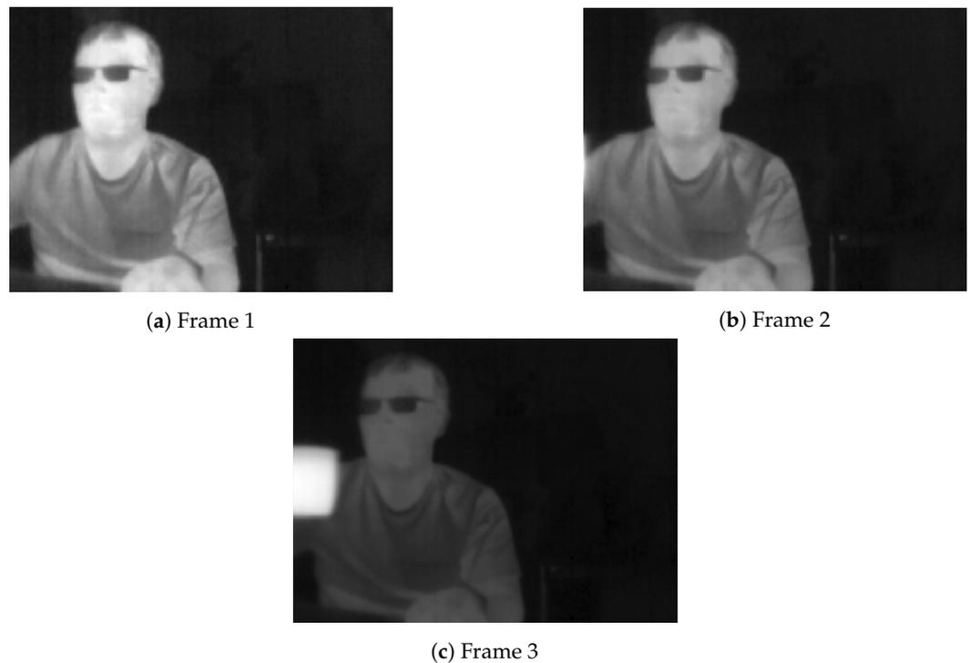
**Figure 3.** Change of contrast caused by AGC when a hot object moves into a scene.
