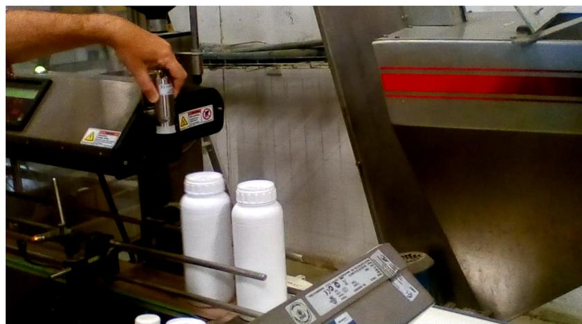
**Figure 13.** Picture taken in the production line during a stop. It shows two bottles right after they passed below the thermal camera. The human hand is adjusting the thermal camera.
