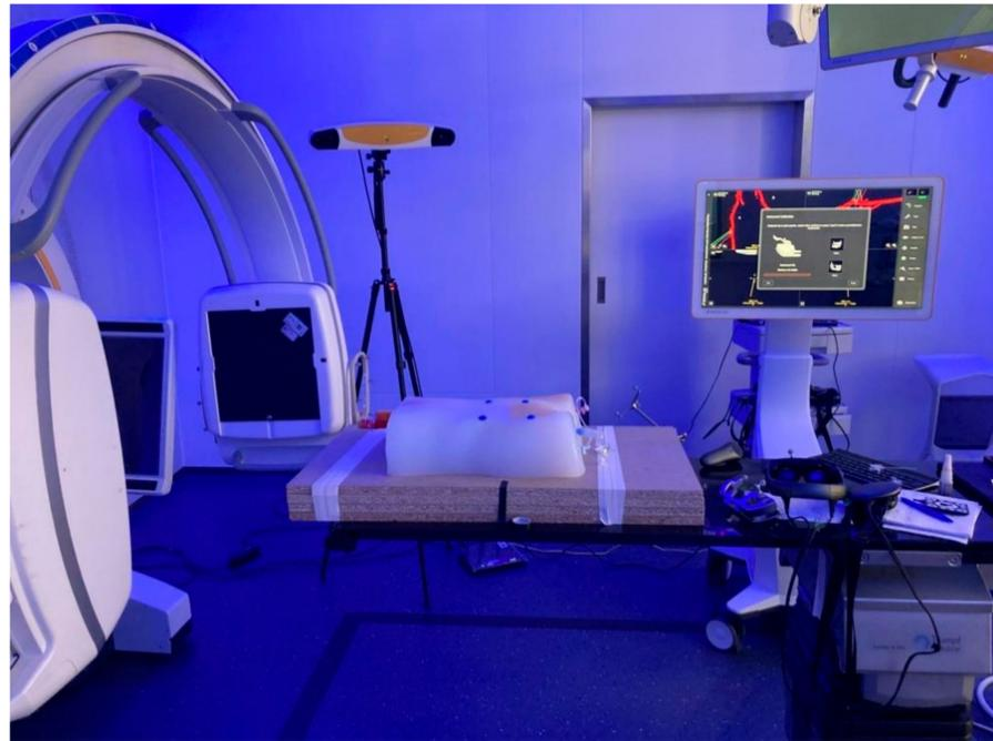
**Figure 3.** Experimental set-up: Phantom model (center), X-ray device (Siemens Cios alpha C-arm, Siemens Healthcare GmbH, Erlangen, Germany) for cone-beam CTA (left), Curve<sup>®</sup> Navigation system (Brainlab AG, Munich, Germany) for optical tracking with tripod camera system and workstation (background), and HMD on the O.R. table (right).
